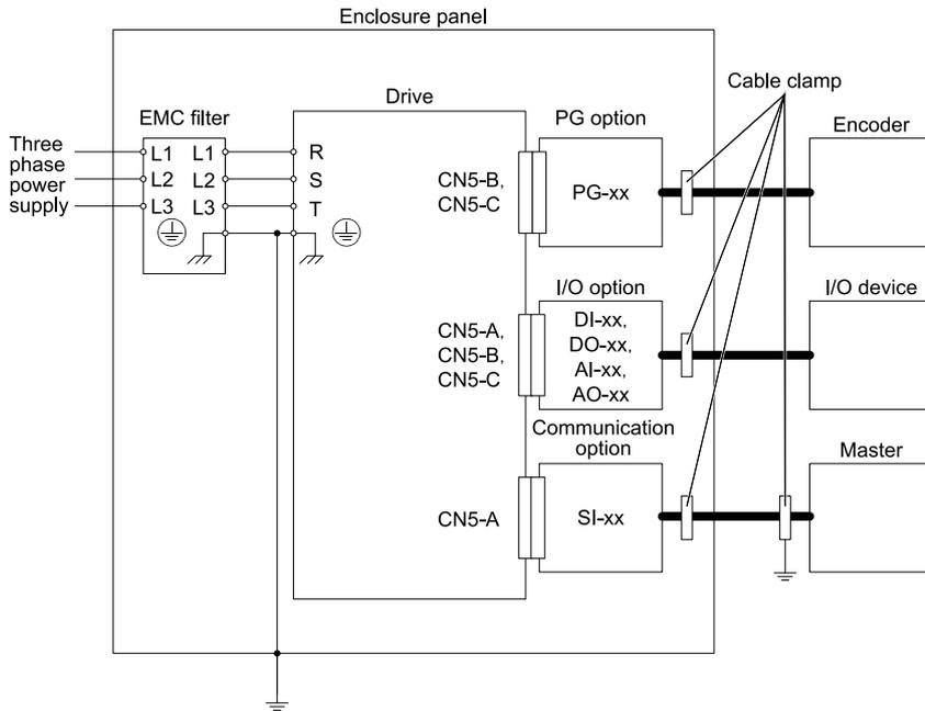
**Figure 12.3 Option Installation for CE Compliance: 1000-Series, GA700, GA800, CR700, CH700**
