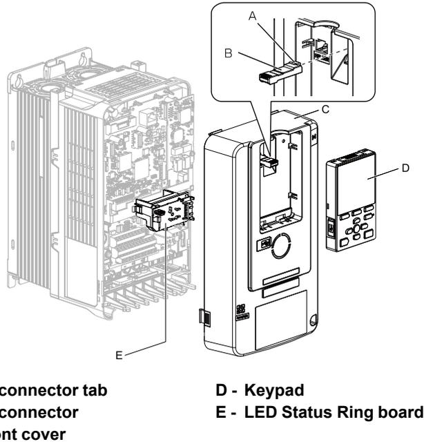
**Figure 5.13 Replace the Front Cover and Keypad**
