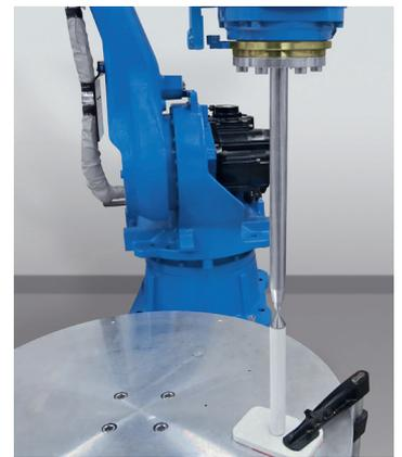
With the calibration tips from Yaskawa we offer a very simple tried and tested tool for a wide range of tasks in your robot system. Due to the rotational symmetry and the manually adjustable length of a calibration tip, a TCP (Tool Center Point) can be set up very simply. Deviations and errors are thereby reduced. The handling and application doesn't require any further training or reading of a manual. The benefit is obvious or depends on the robot flange.
