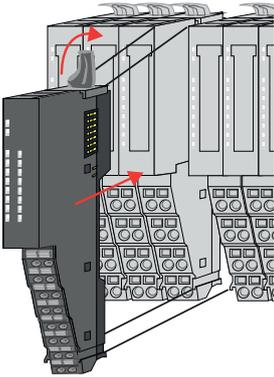
6. ➤ To mount the module put it to the gap between the both modules and push it, guided by the stripes at both sides, to the profile rail.
