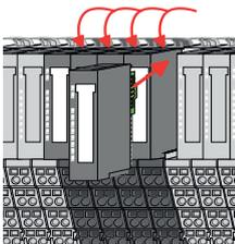
9. Plug again the electronic module, which you have removed before.
