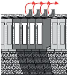
4. Turn all the locking lever of the module group to be exchanged upwards.
