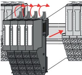
7. To mount the module group put it to the gap between the both modules and push it, guided by the stripes at both sides, to the profile rail.
