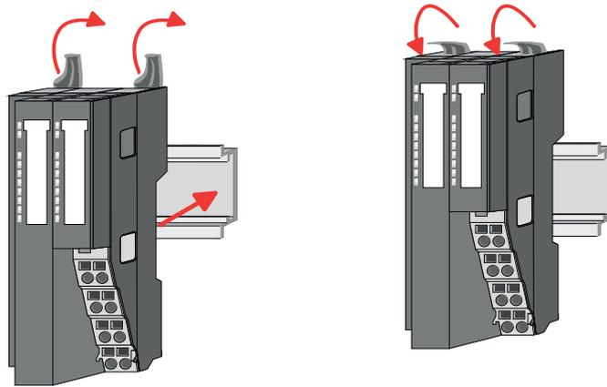
2. → Turn the locking lever upwards, place the bus coupler at the profile rail and turn the lever downward.
