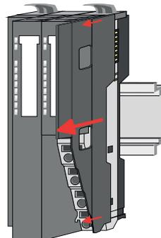
1. → Before mounting the periphery modules you have to remove the bus cover at the right side of the bus coupler by pulling it forward. Keep the cover for later mounting.
