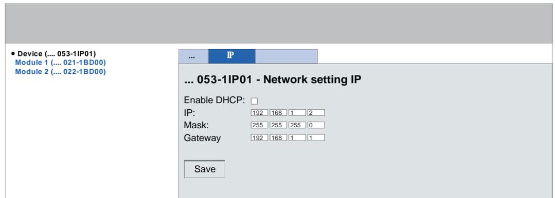
2. → Enter the relevant IP address data here. Press [Save] to accept the entries.
