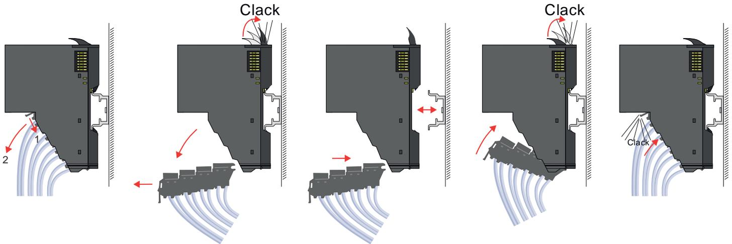
**Exchange of a 16x periphery module**
