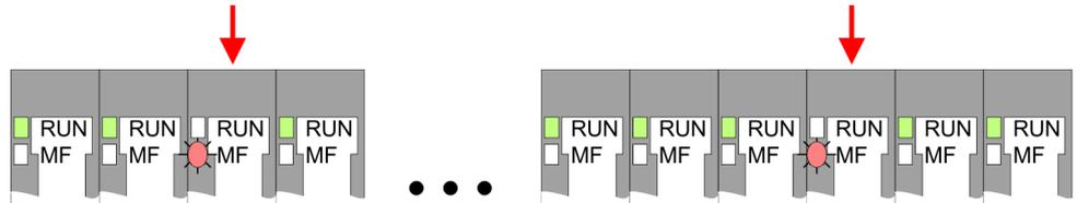
**Behavior:** After PowerON the MF LED of one module respectively more modules flashes. The RUN LED remains off.
