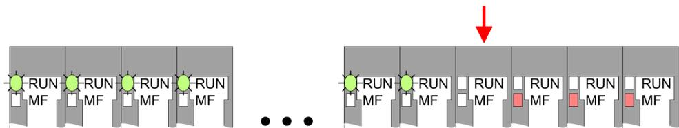
**Behavior:** After PowerON all of the RUN LEDs up to the defective module are flashing. With all following modules the MF LED is on and the RUN LED is off.
