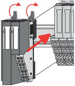
6. → For mounting turn all the locking lever of the bus coupler to be exchanged upwards.
