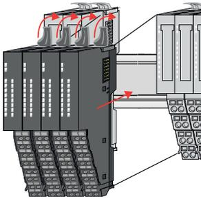
6. ➤ To mount the module group put it to the gap between the both modules and push it, guided by the stripes at both sides, to the profile rail.
