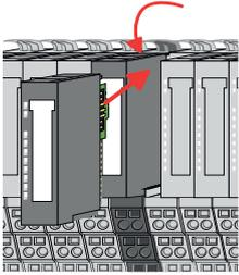
9. Plug again the electronic module, which you have removed before.
