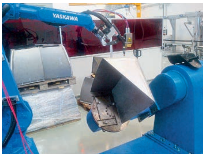
Seamtracking with MIG/MAG torch
