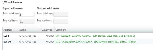
Here you have a list of addresses that are used by the module in the address area of the CPU. By entering a new 'Start address' you can adjust the addressing of the input and output areas accordingly. You can edit 'Name' and 'Comment' by clicking at the corresponding entry.
