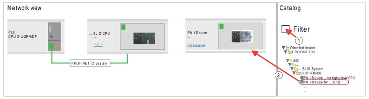
2. To connect to the CPU, click at 'not assigned' and select the PROFINET interface of the CPU.
