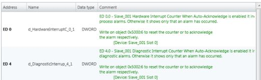
Here you have a list of addresses that are used by the I/O components of all the modules in the address area of the CPU. By entering a new 'Start address' you can adjust the addressing of the input and output areas accordingly. You can edit 'Name' and 'Comment' by clicking at the corresponding entry.
