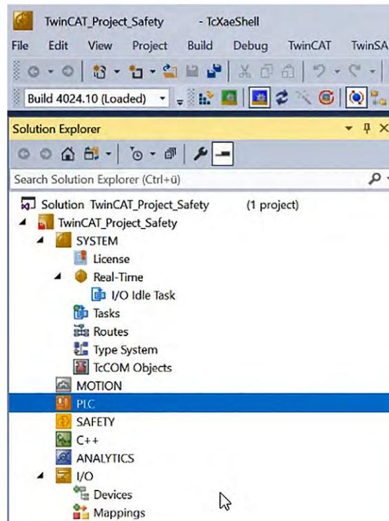
Fig. 69: TwinCAT 3 - PLC and SAFETY are separated items
