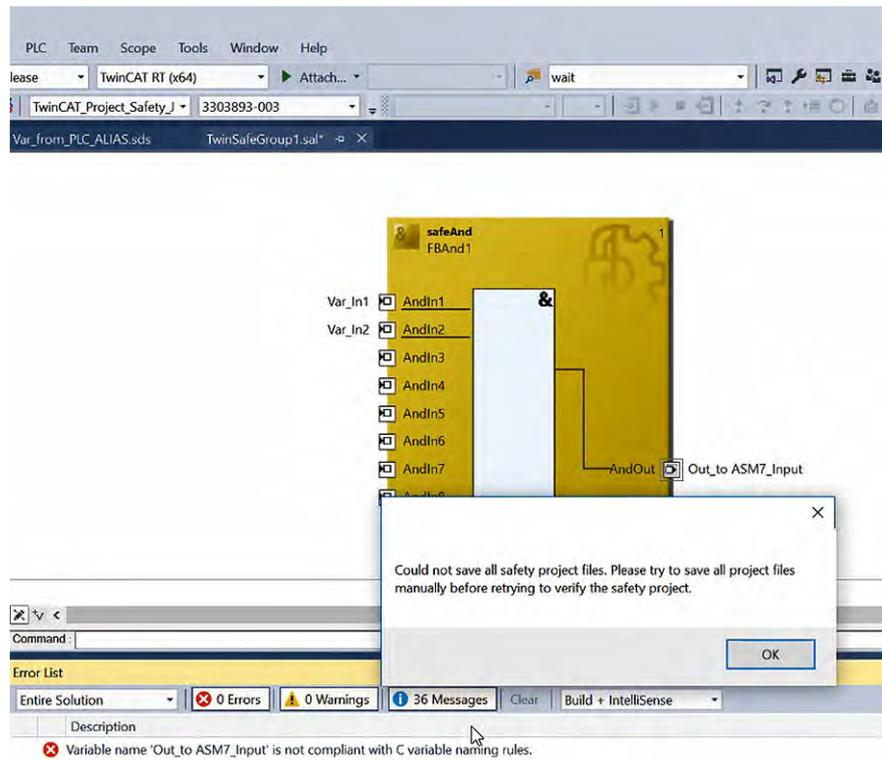
Fig. 143: TwinCAT 3 - Verify Safety Project - Could not save all safety project files
