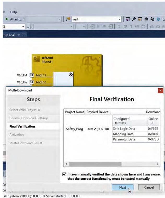
Fig. 148: TwinCAT 3 - Final Verification
