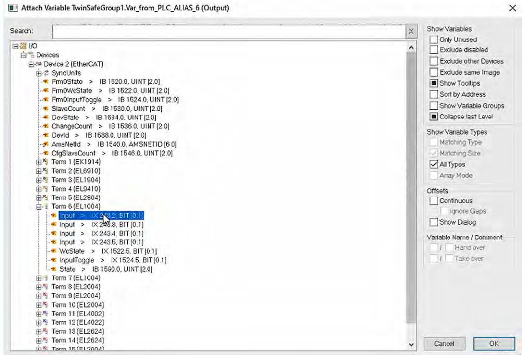
Fig. 134: TwinCAT 3 - Link Var\_from\_PLC\_ALIAS to EL1004
