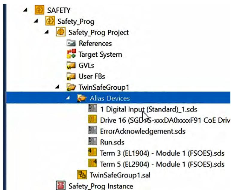
Fig. 127: TwinCAT 3 - Digital Input as Alias Device in TwinSafeGroup1 added
