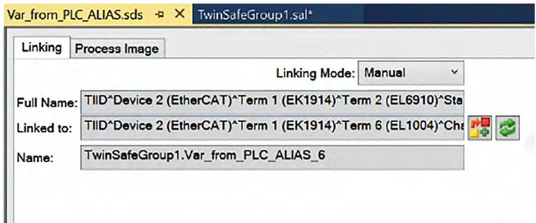
Fig. 135: TwinCAT 3 - Var\_from\_PLC\_ALIAS linked to input of EL1004
