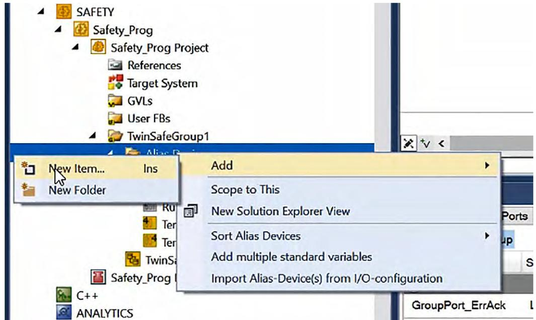
Fig. 125: TwinCAT 3 - Add Alias Device in TwinSafeGroup1
