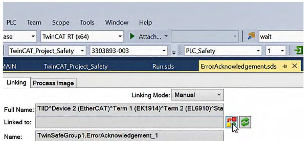
Fig. 101: TwinCAT 3 - ErrorAcknowledgement - Link Button
