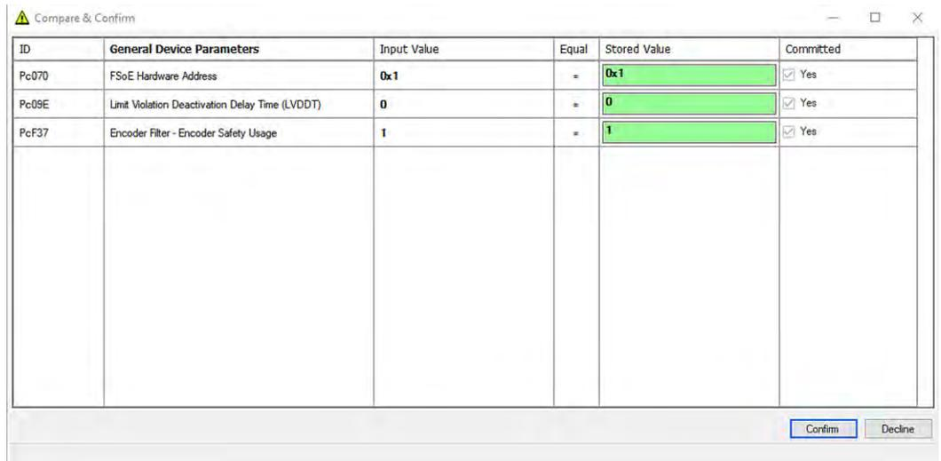
Fig. 45: Compare & Confirm General Device Parameters
