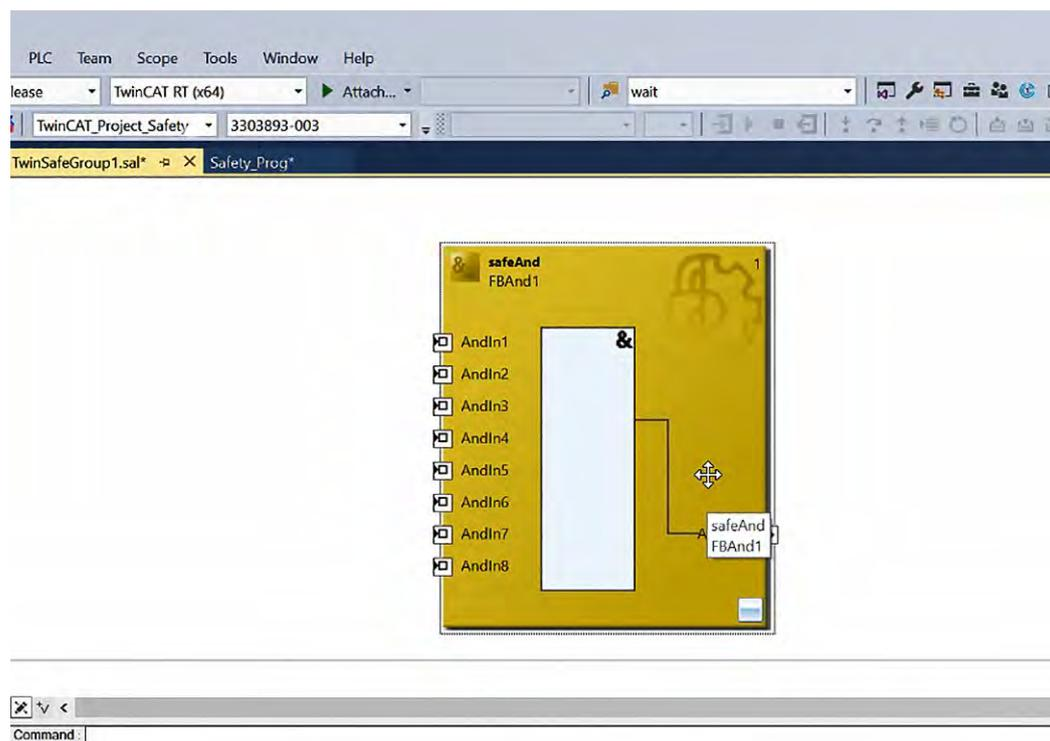
Fig. 114: TwinCAT 3 - safeAnd dropped in TwinSafeGroup1
