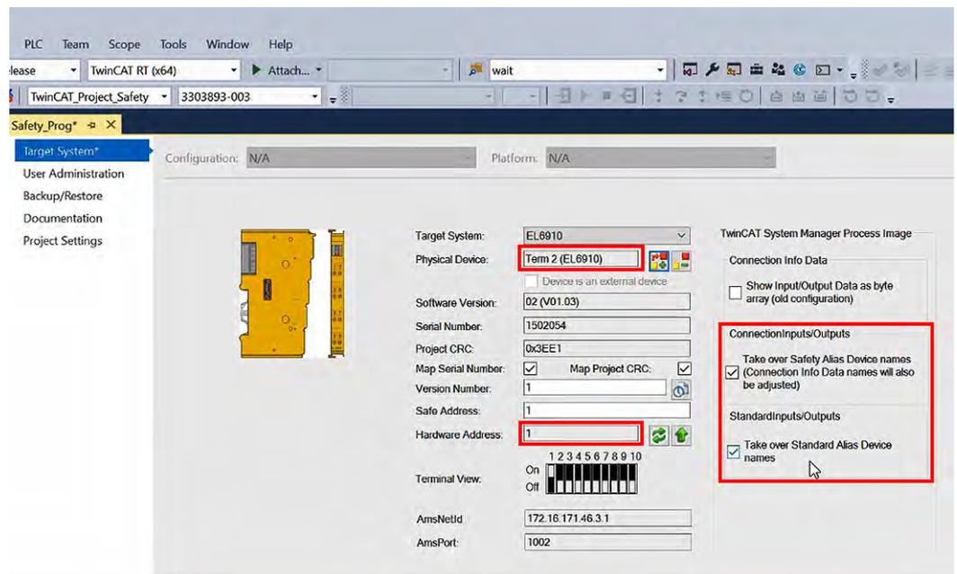
Fig. 83: TwinCAT 3 - Physical device is mapped
