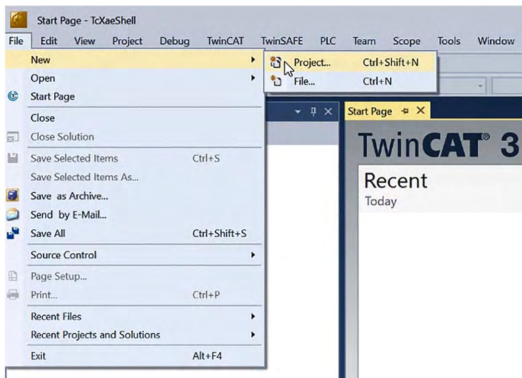
Fig. 65: TwinCAT 3 - Create new project
