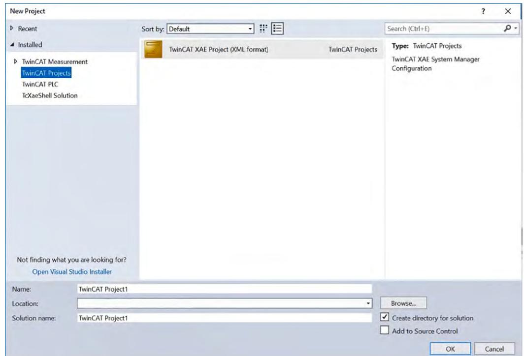
Fig. 66: TwinCAT 3 - Create new project - Select TwinCAT XAE Project
