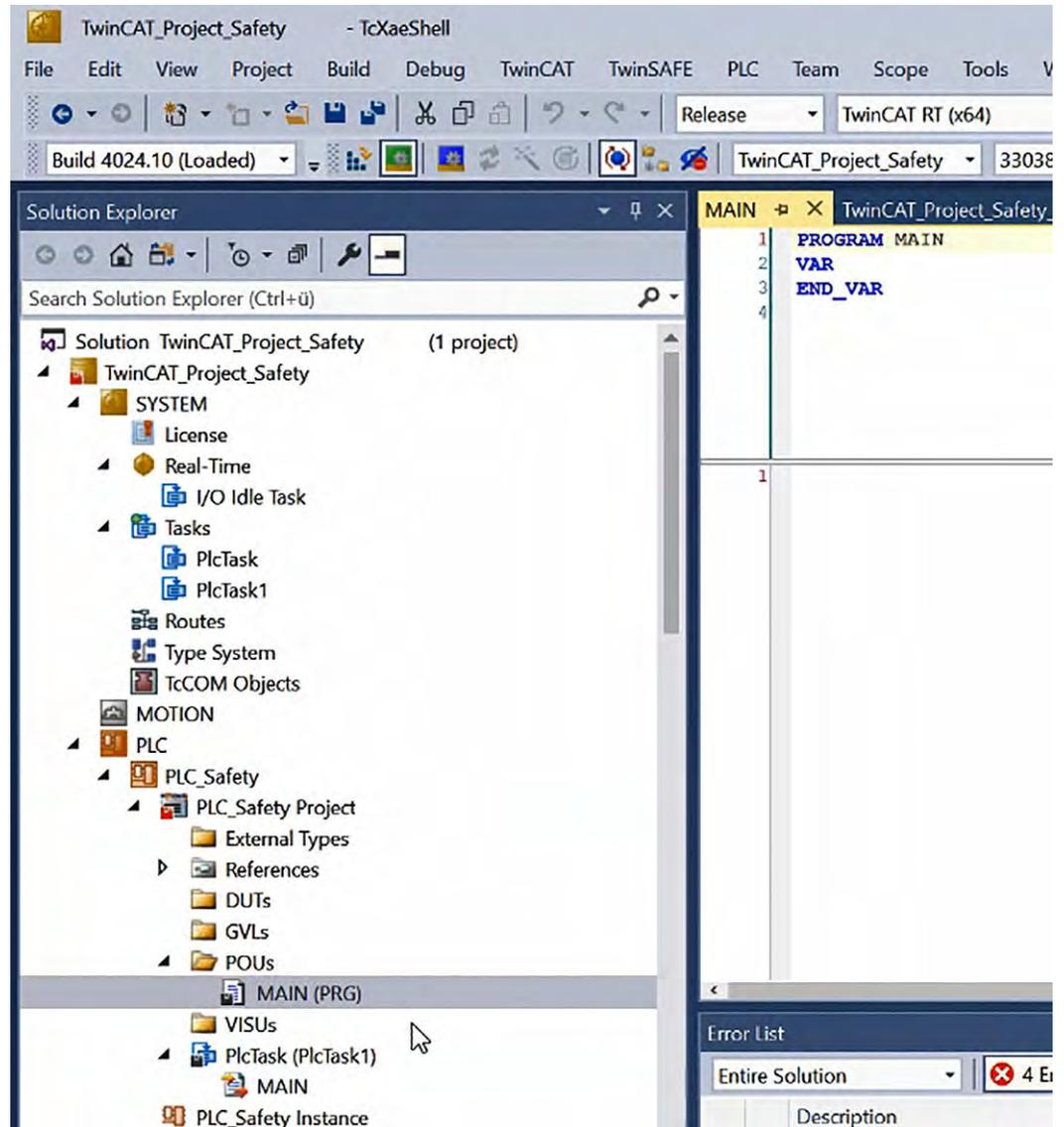
Fig. 94: TwinCAT 3 - Open MAIN PLC program
