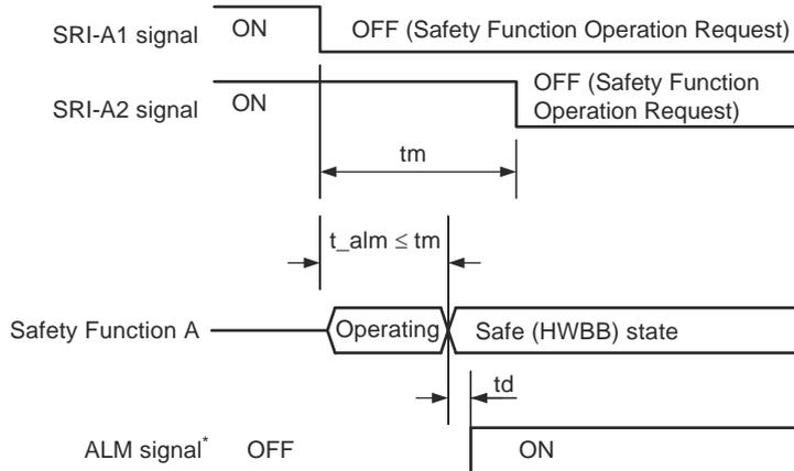
Fig. 157: Input behaviour of SGDV-OSA01A
