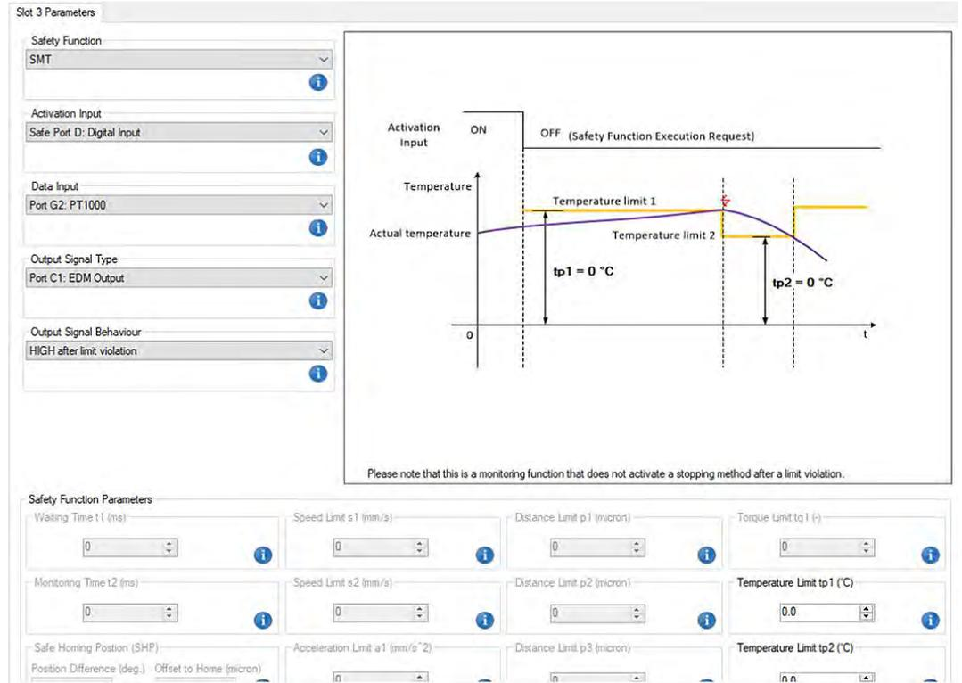
Fig. 32: Completed Slot 3 Parameters dialog
