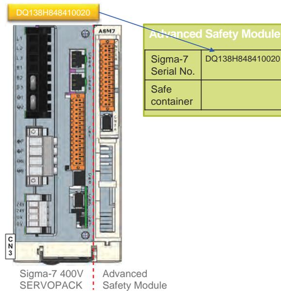
Fig. 5: Pairing of Safety Module and SERVOPACK
