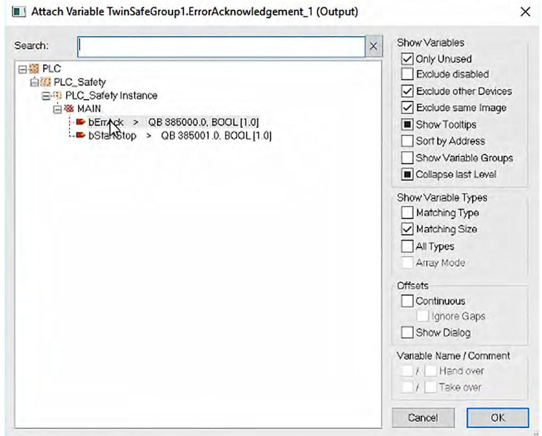
Fig. 102: TwinCAT 3 - Attach Variable `bErrAck` to ErrorAcknowledgement
