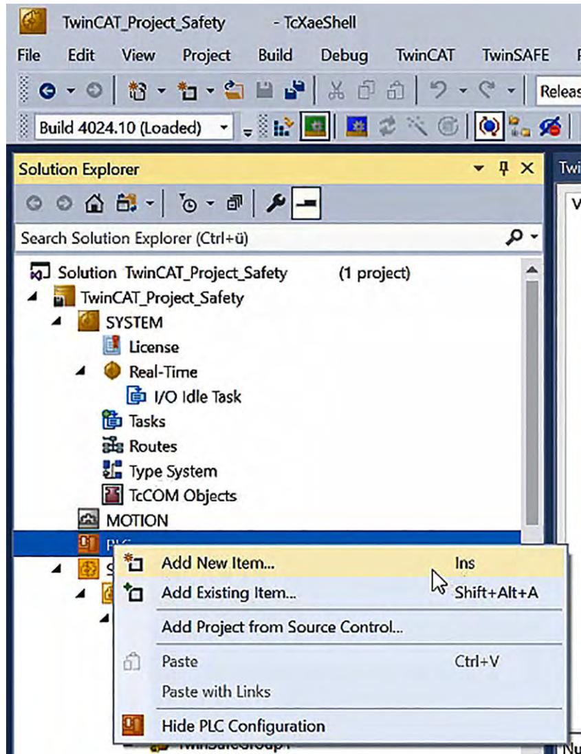
Fig. 91: TwinCAT 3 - Add New Item in PLC
