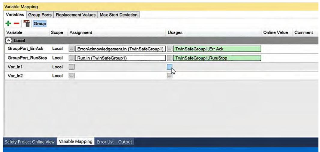
Fig. 116: TwinCAT 3 - Open *Usage Map to* dialog for variable *Var\_In1*
