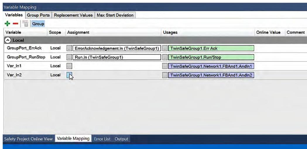
Fig. 121: TwinCAT 3 - Open Assignment Map to dialog for variable *Var\_In2*
