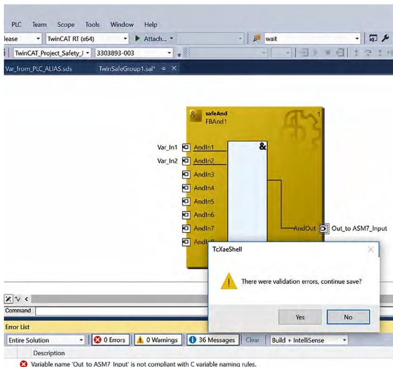
Fig. 142: TwinCAT 3 - Verify Safety Project - There were validation errors
