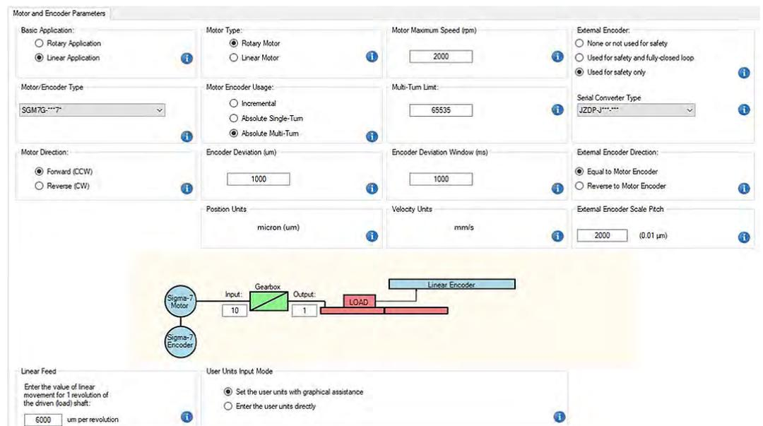
Fig. 24: Motor and Encoder Parameters dialog
