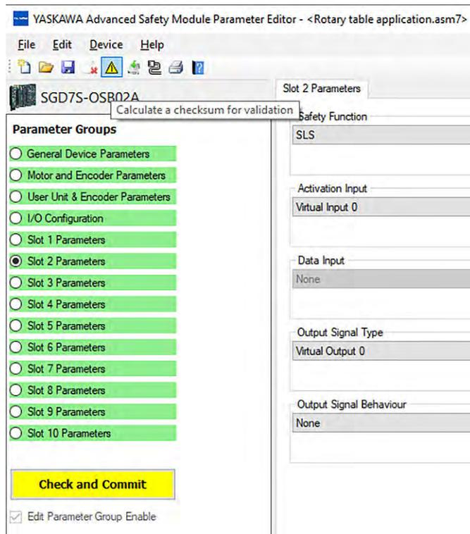
Fig. 54: Calculate a Checksum for Validation
