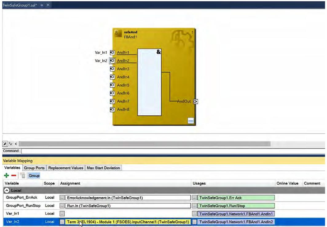
Fig. 123: TwinCAT 3 - Variable *Var\_In2* assigned to *InputChannel1* of *EL1904*
