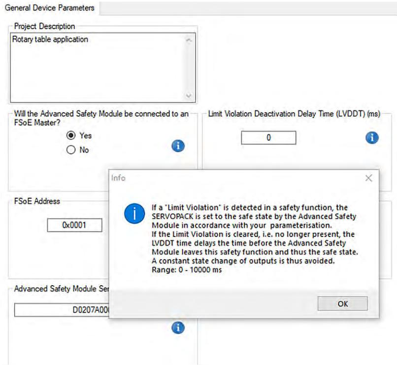
Fig. 44: Limit Violation Deactivation Delay Time Help Text
