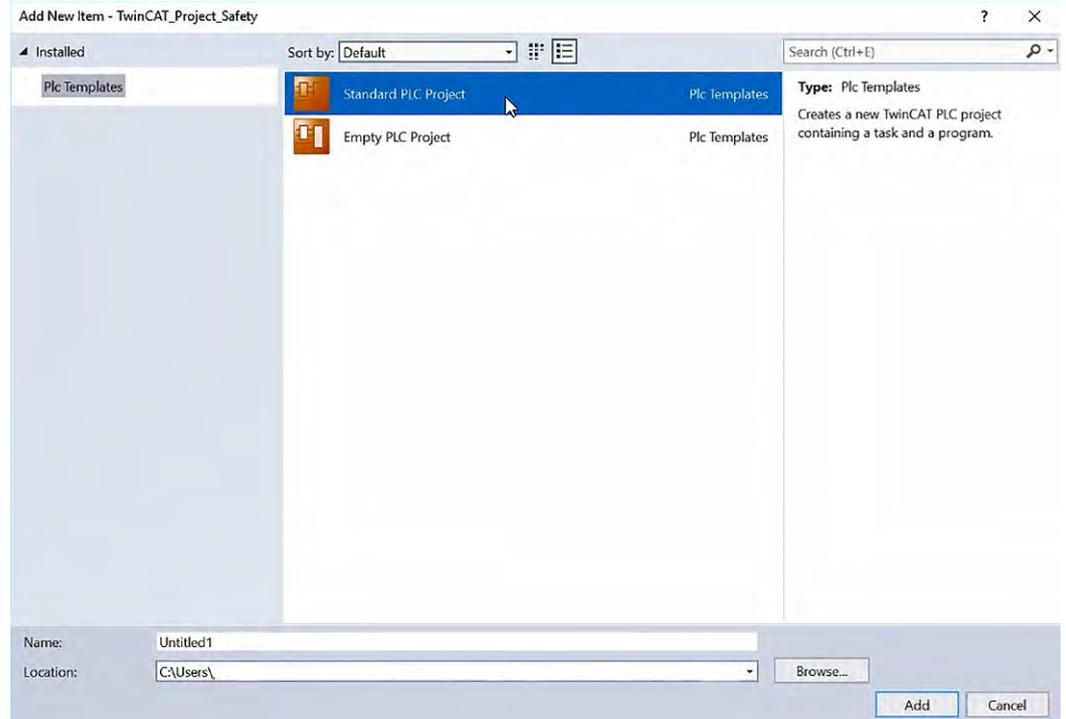
Fig. 92: TwinCAT 3 - Create Standard PLC Project
