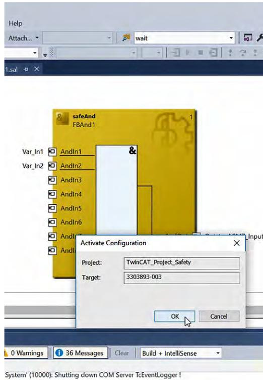
Fig. 152: TwinCAT 3 - Confirm Activation
