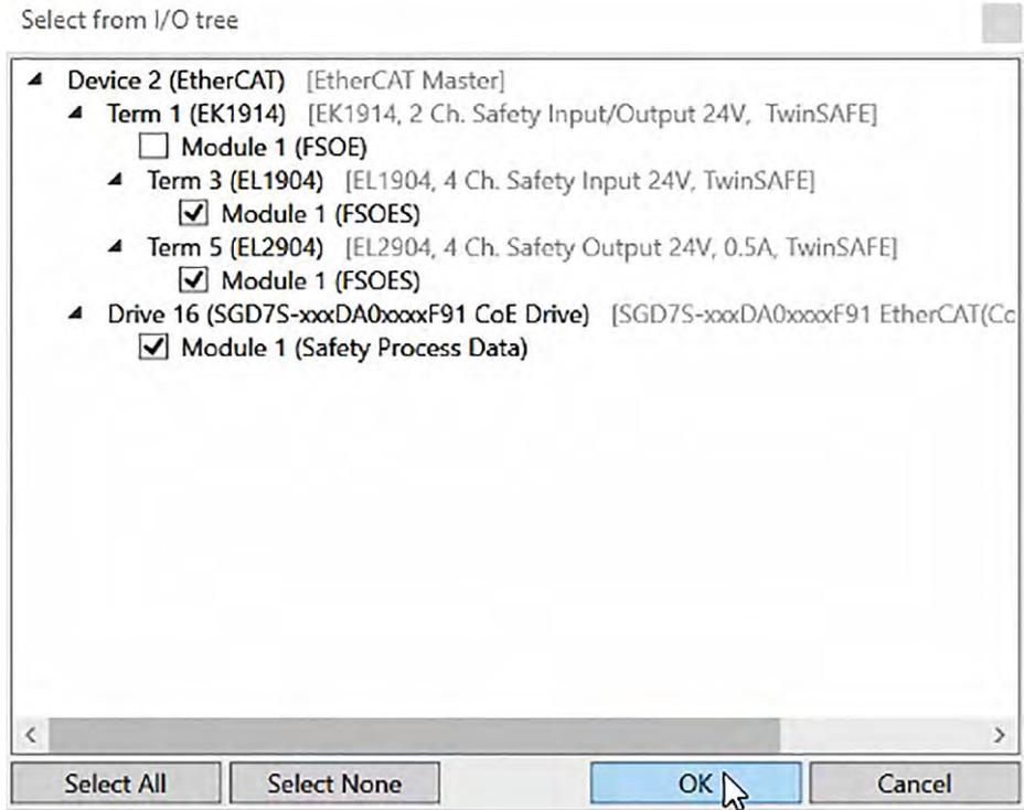
Fig. 86: TwinCAT 3 - Select Alias Devices from IO tree
