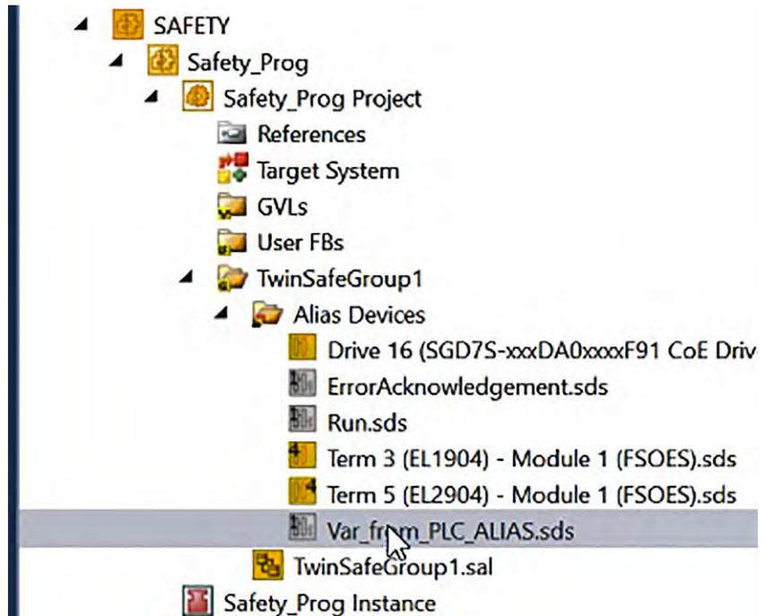
Fig. 132: TwinCAT 3 - Open `Var_from_PLC_ALIAS` in *Solution Explorer*
