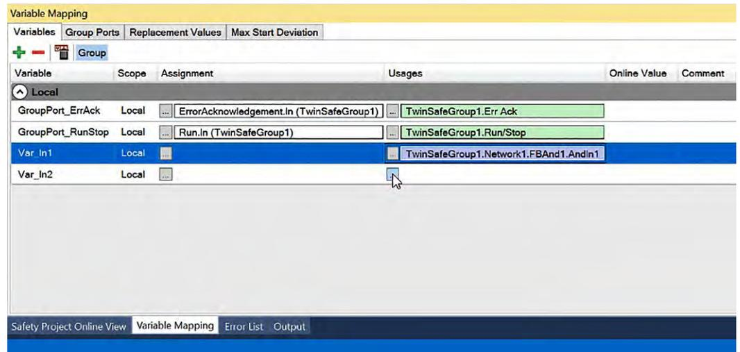
Fig. 118: TwinCAT 3 - Open Usage Map to dialog for variable *Var\_In2*
