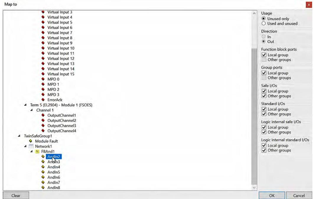
Fig. 119: TwinCAT 3 - Map Usage to AndIn2 for variable Var\_In2
