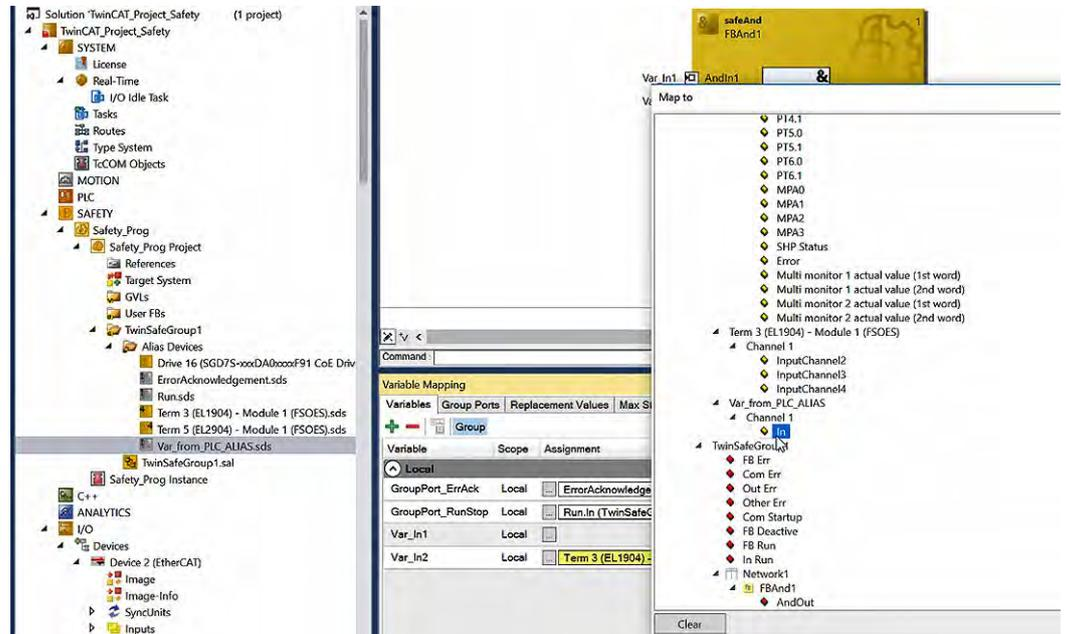
Fig. 130: TwinCAT 3 - Assign *Var\_In1* to *Var\_from\_PLC\_ALIAS*
