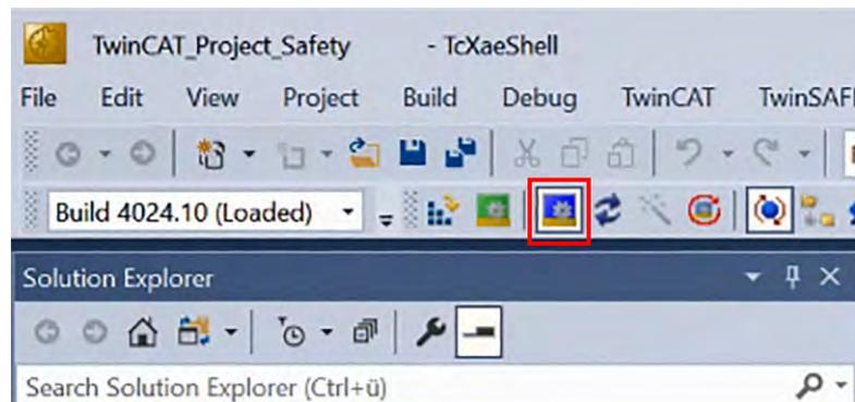
Fig. 68: TwinCAT 3 - Restart TwinCAT (Config Mode)
