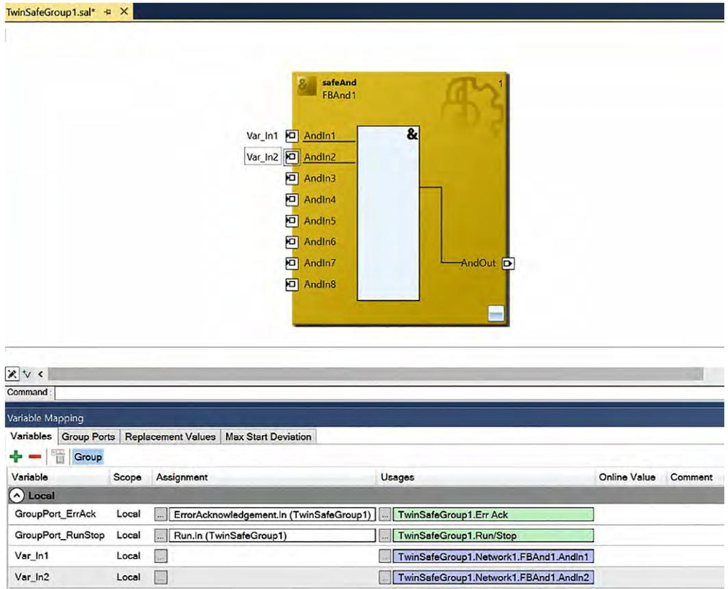
Fig. 120: TwinCAT 3 - Variable Var\_In1 and Var\_In2 linked to safeAnd
