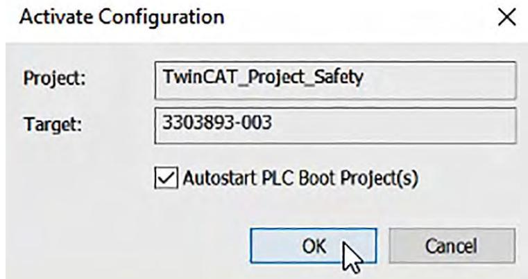
Fig. 98: TwinCAT 3 - Activate Configuration Dialog box
