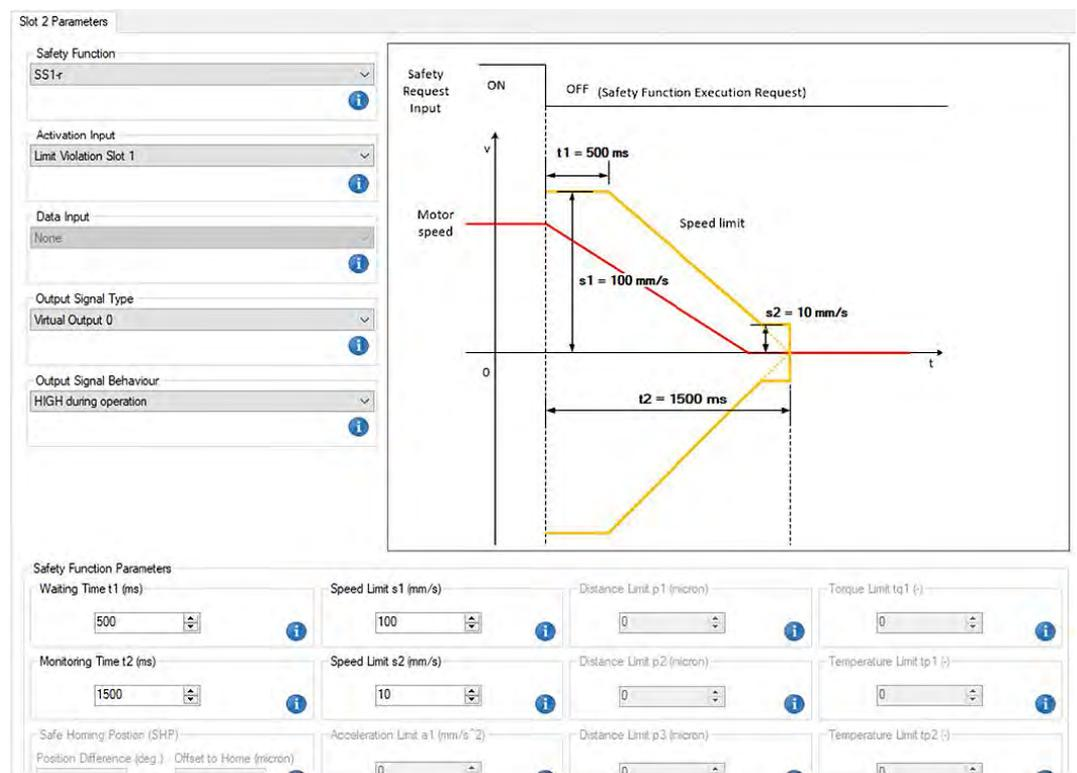
Fig. 30: Completed Slot 2 Parameters dialog
