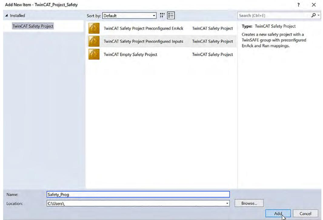
*Fig. 78: TwinCAT 3 - SAFETY - Add New Item - Select TwinCAT Safety Project Preconfigured Inputs - Create Safety Project*
