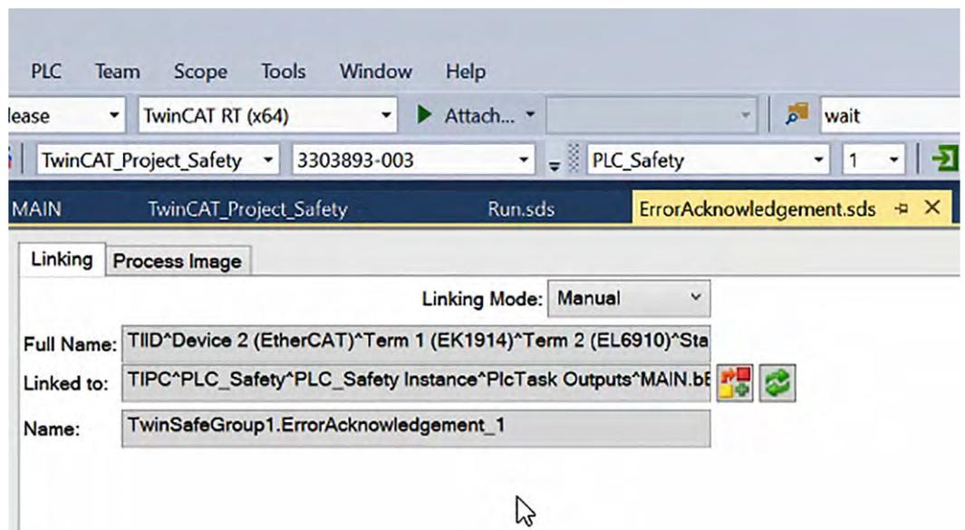
Fig. 103: TwinCAT 3 - Variable `bErrAck` attached to ErrorAcknowledgement
