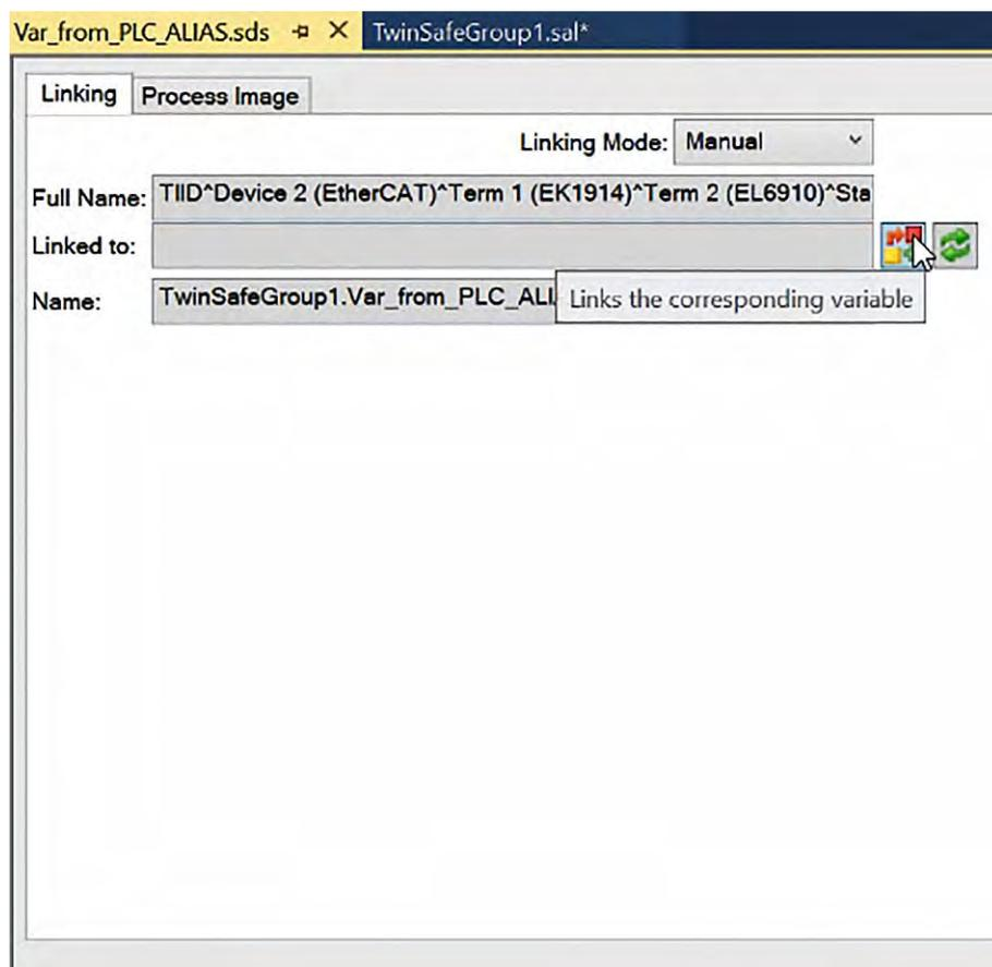
Fig. 133: TwinCAT 3 - Link Button of Var\_from\_PLC\_ALIAS
