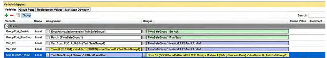
Fig. 140: TwinCAT 3 - Out\_to\_ASM7\_Input assigned to Advanced Safety Module
