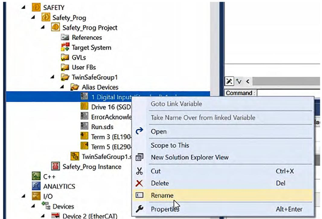
Fig. 128: TwinCAT 3 - Rename added Digital Input in TwinSafeGroup1
