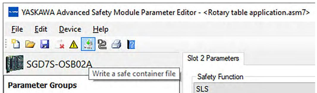
Fig. 55: Write a Safe Container File
