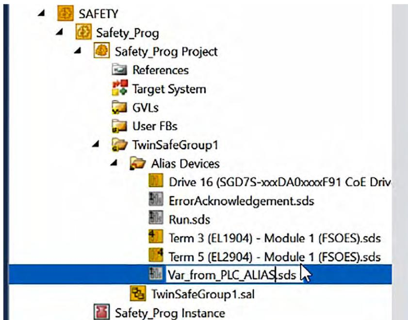
Fig. 129: TwinCAT 3 - Digital Input in TwinSafeGroup1 renamed as Var\_from\_PLC\_ALIAS
