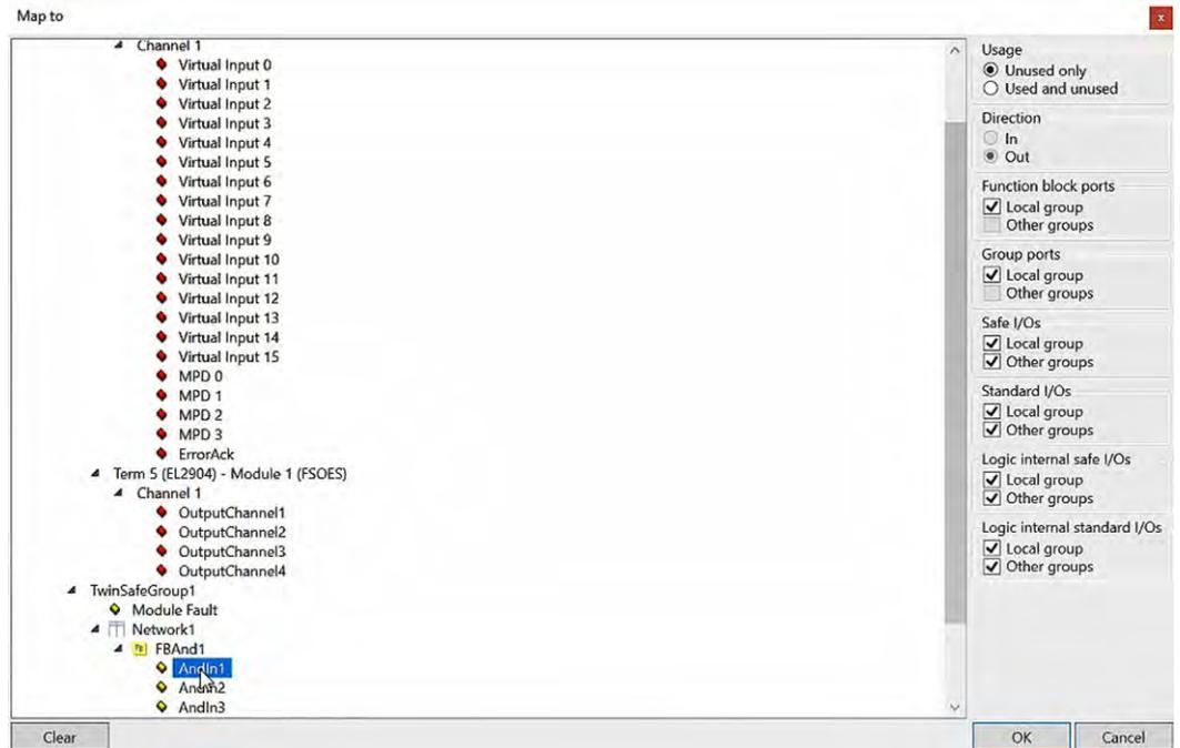
Fig. 117: TwinCAT 3 - Map Usage to *AndIn1* for variable *Var\_In1*
