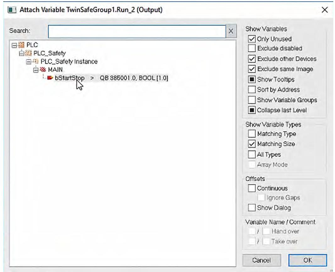
Fig. 106: TwinCAT 3 - Attach Variable `bStartStop` to Run
