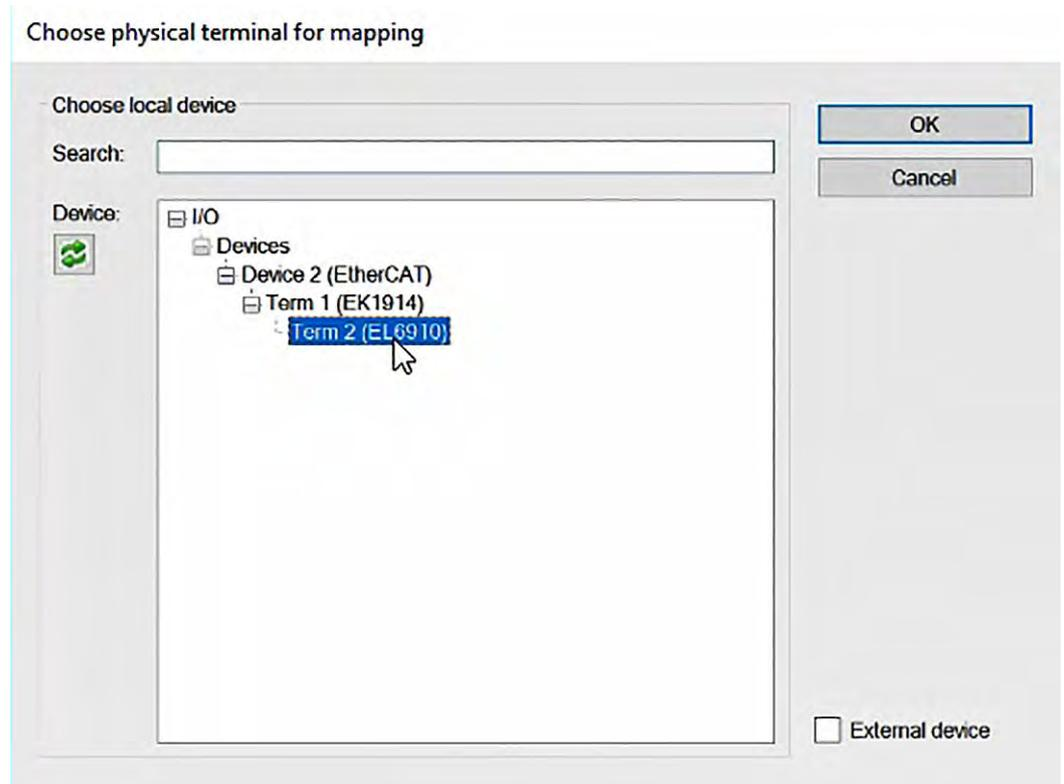
Fig. 82: TwinCAT 3 - Choose physical terminal for mapping
