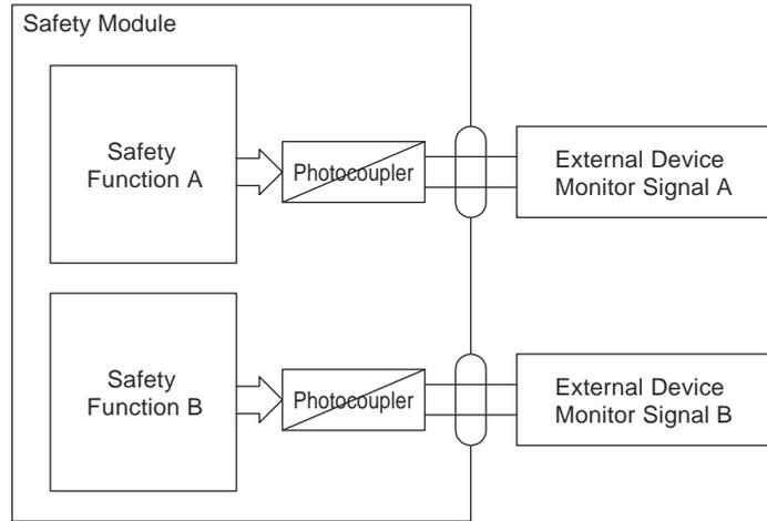
Fig. 159: Relationship between the External Device Monitor Signal and safety function
