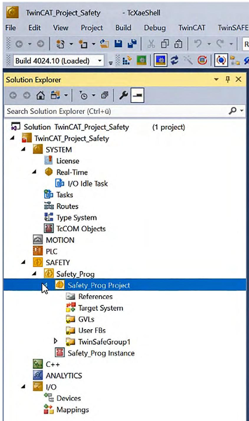
Fig. 80: TwinCAT 3 - Safety Project is created in the Solution Explorer
