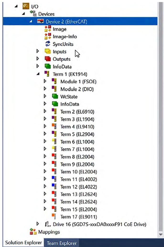
Fig. 75: TwinCAT 3 - Found devices after scanning for boxes
