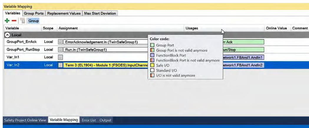
Fig. 124: TwinCAT 3 - Color code for variable mapping
