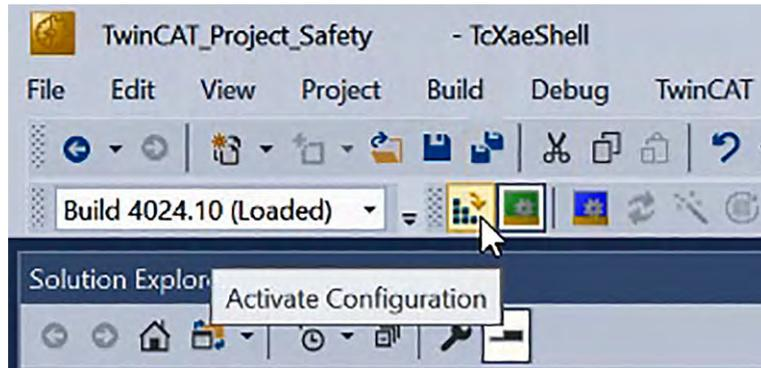
Fig. 97: TwinCAT 3 - Activate Configuration
