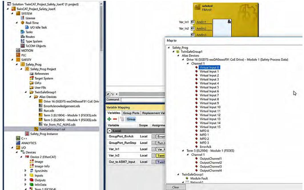
Fig. 139: TwinCAT 3 - Assign Virtual Input 1 to Advanced Safety Module
