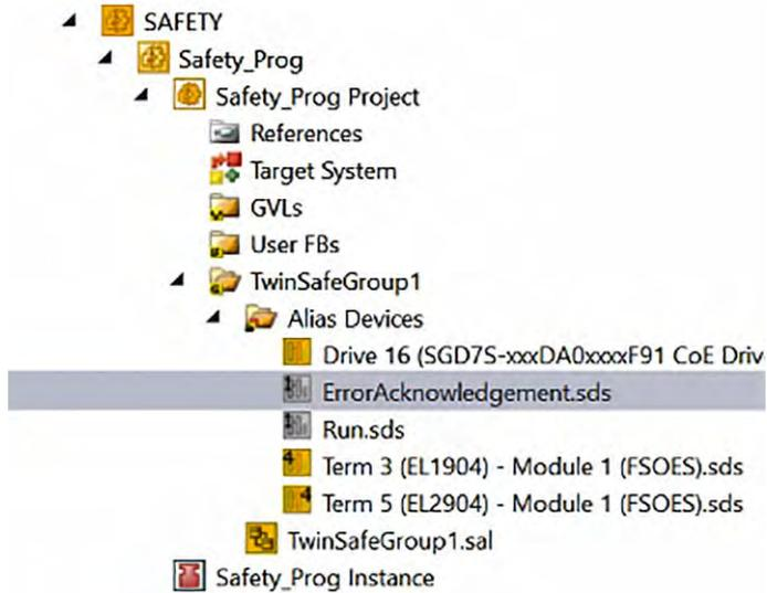
Fig. 100: TwinCAT 3 - ErrorAcknowledgement Alias Device in Solution Explorer
