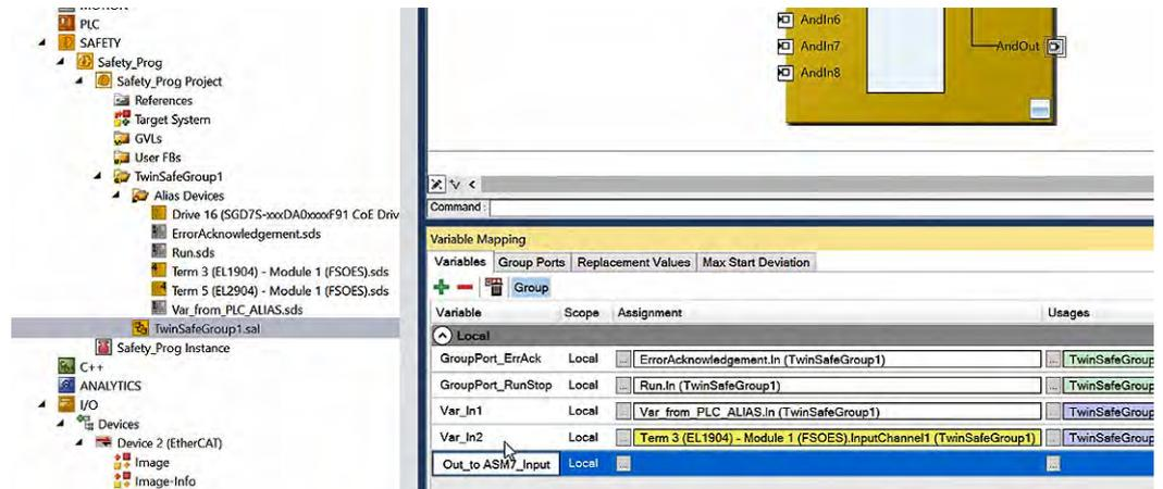
Fig. 136: TwinCAT 3 - Create variable *Out\_to\_ASM7\_Input* in *TwinSafeGroup1*
