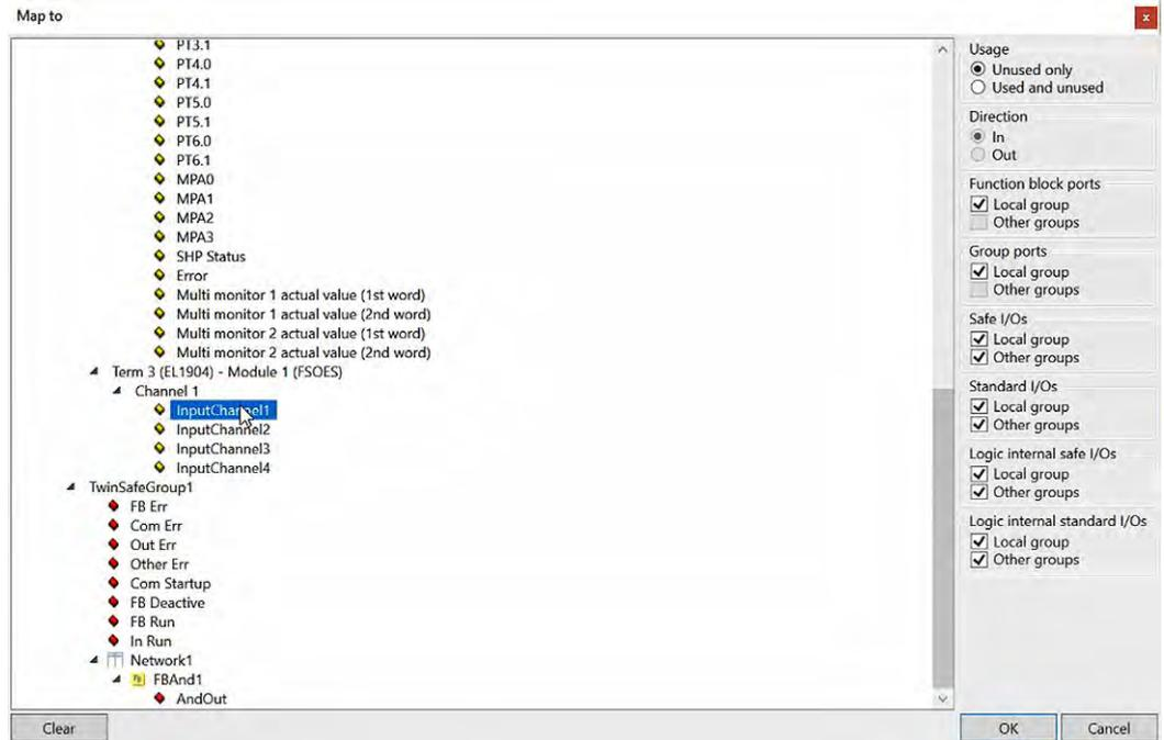
Fig. 122: TwinCAT 3 - Map variable *Var\_In2* to *InputChannel1* of *EL1904*
