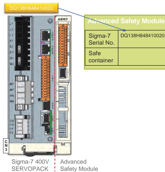
Fig. 1: Pairing of Safety Module and SERVOPACK
