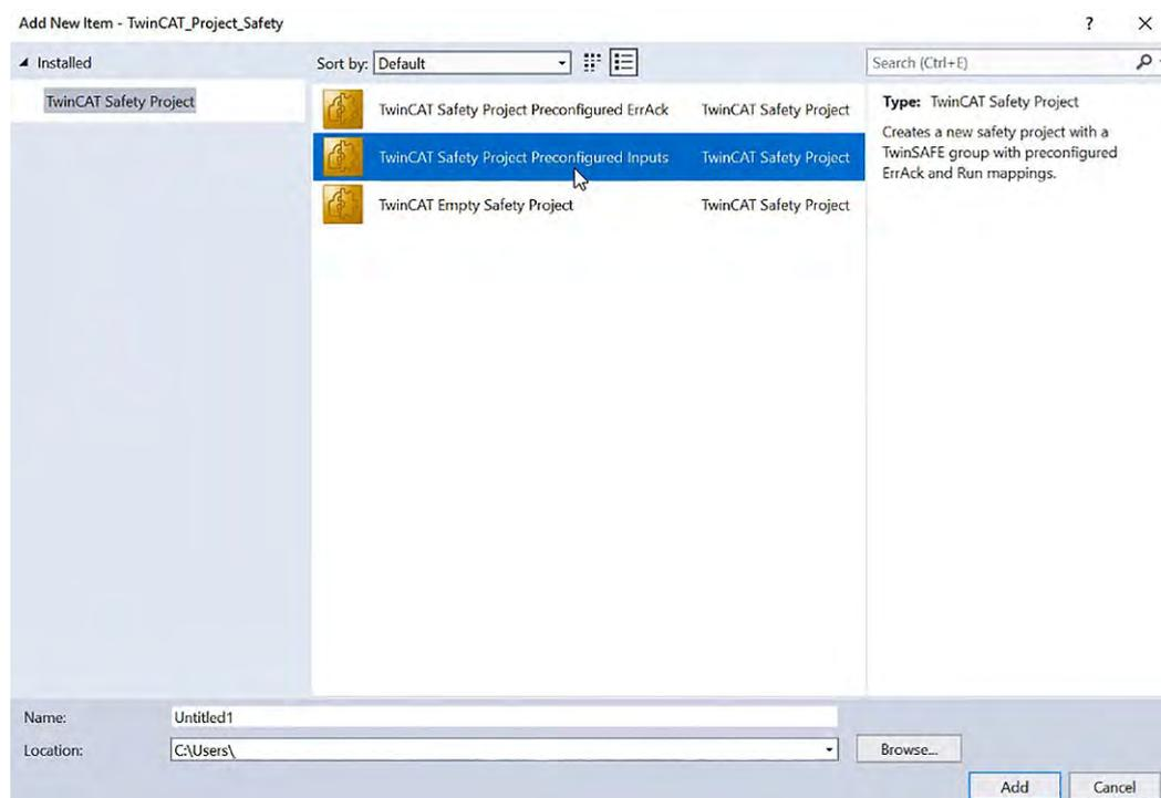
*Fig. 77: TwinCAT 3 - SAFETY - Add New Item - Select TwinCAT Safety Project Preconfigured Inputs*
