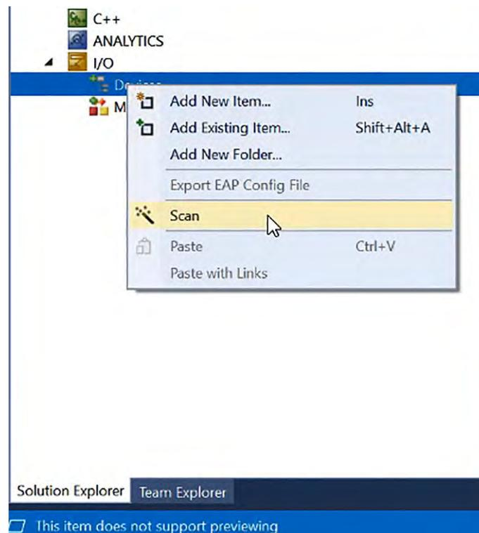
Fig. 71: TwinCAT 3 - Scan Hardware configuration
