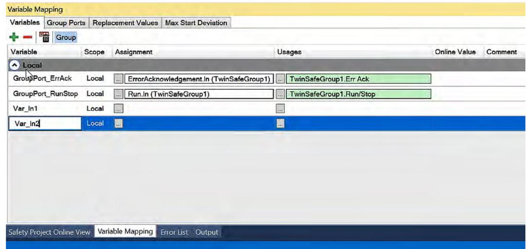
Fig. 115: TwinCAT 3 - Create variables *Var\_In1* and *Var\_In2* for *safeAnd*
