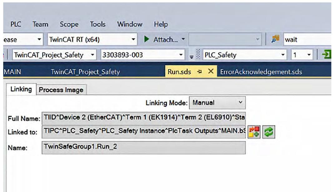
Fig. 107: TwinCAT 3 - Variable `bStartStop` attached to Run
