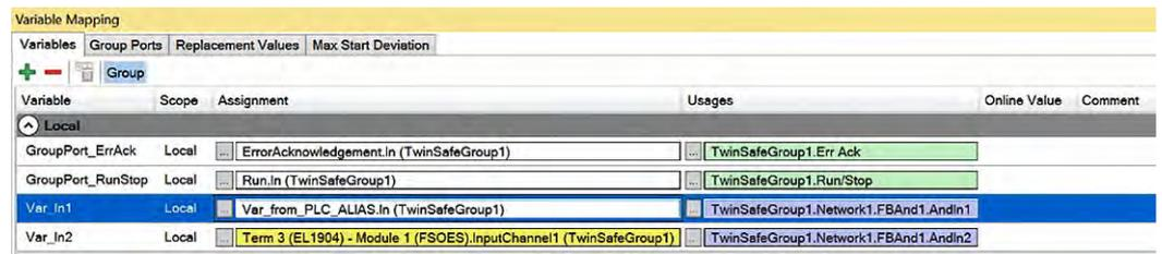
Fig. 131: TwinCAT 3 - *Var\_from\_PLC\_ALIAS* assigned to *Var\_In1*
