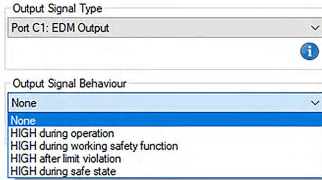
Fig. 163: Output Signal Type and Output Signal Behaviour
