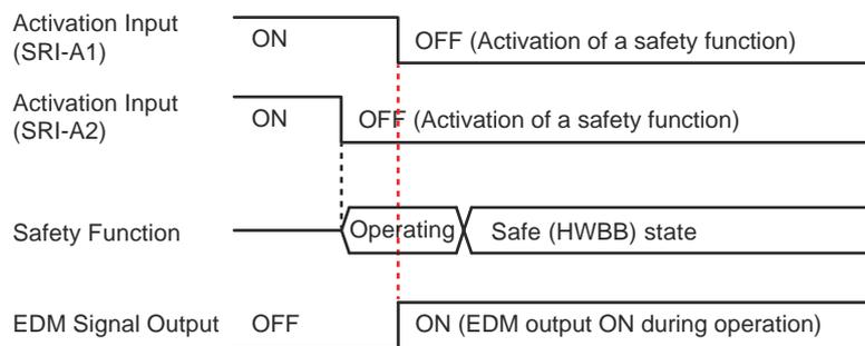
Fig. 164: EDM output behaviour of SGD7S-OSA01A
