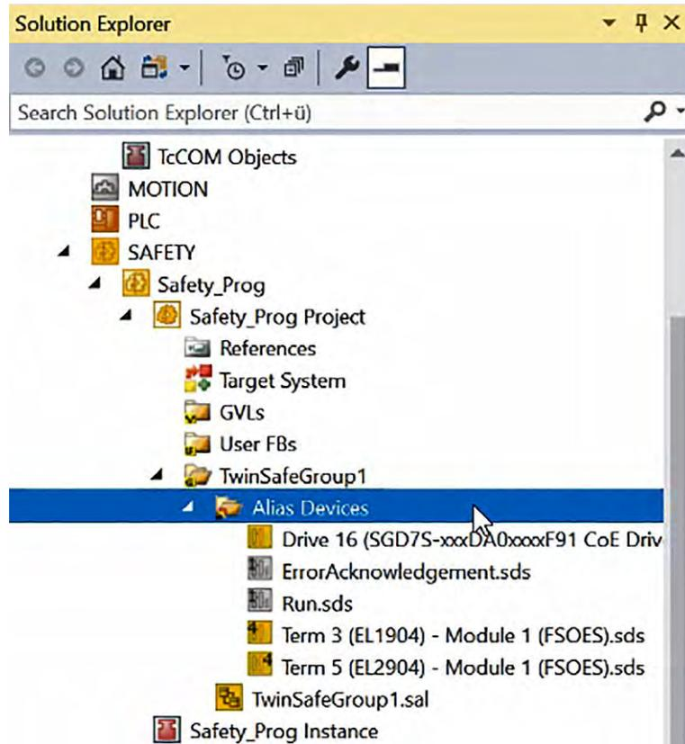
Fig. 88: TwinCAT 3 - Alias Devices in TwinSafeGroup imported
