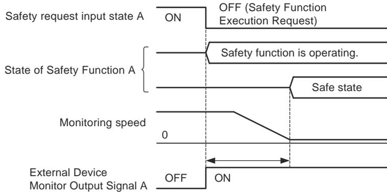
**Fig. 161: Operation Timing When Pc01.0 = 0 (Output Condition = Safety Function Operation)**
