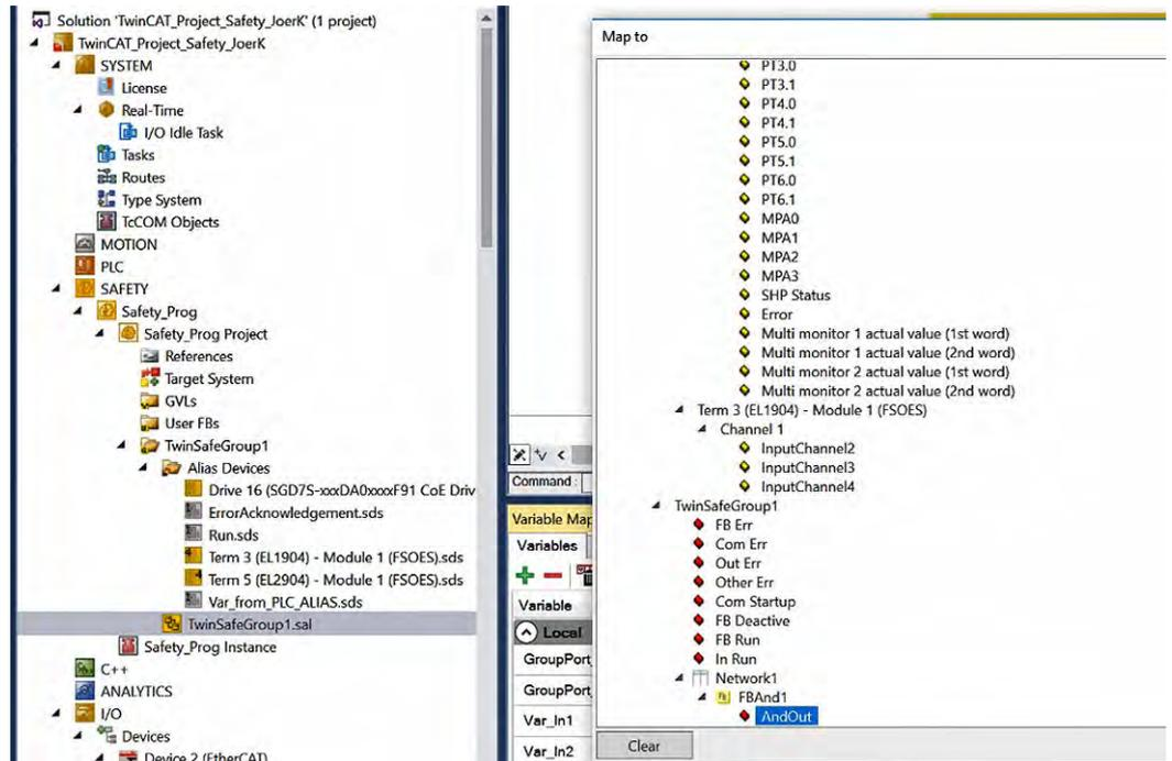
Fig. 137: TwinCAT 3 - Assign *Out\_to\_ASM7\_Input* to *FBAnd1*
