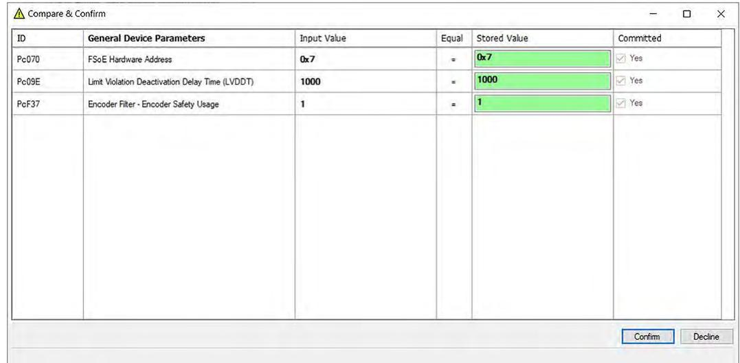
Fig. 22: Compare and Confirm dialog for the General Device Parameters
