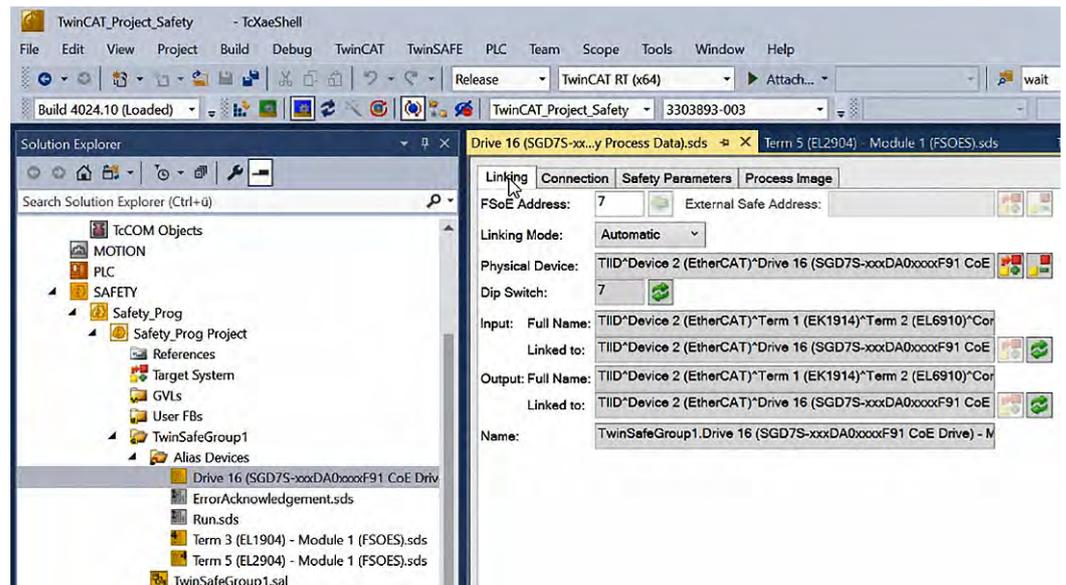
Fig. 90: TwinCAT 3 - Properties of the SGD7S Alias Device
