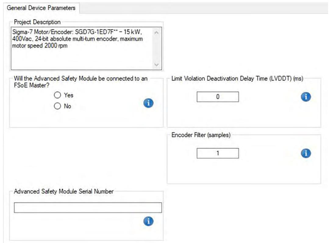
Fig. 20: The General Device Parameters dialog
