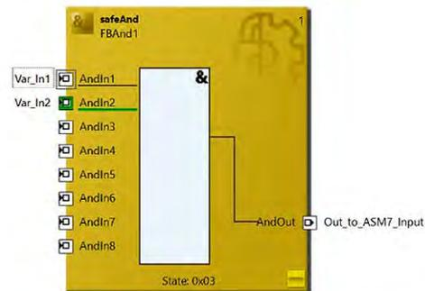
Fig. 156: TwinCAT 3 - Group is in state RUN
