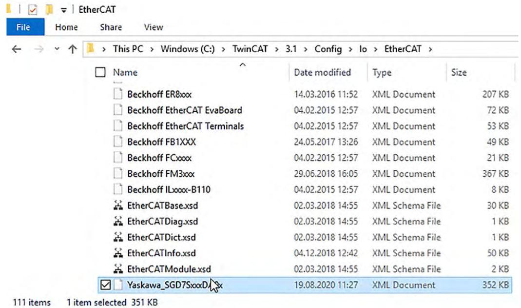
Fig. 70: TwinCAT 3 - Local path for Sigma-7 ESI file
