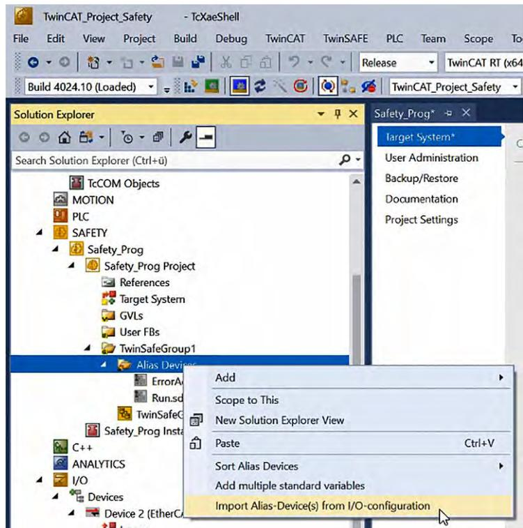
Fig. 85: TwinCAT 3 - Import Alias Device(s) from IO configuration
