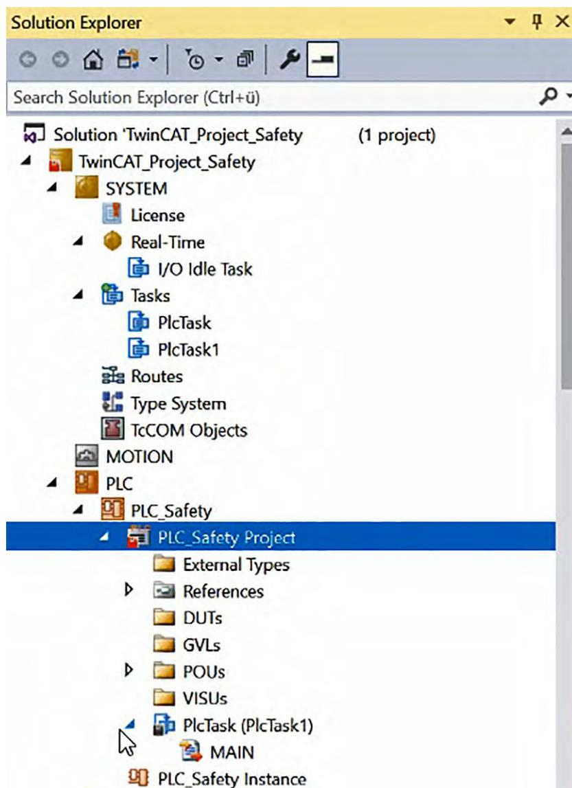
Fig. 93: TwinCAT 3 - Standard PLC Project created
