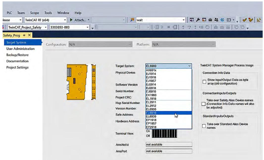
Fig. 81: TwinCAT 3 - Select Target System EL6910 for Safety Project
