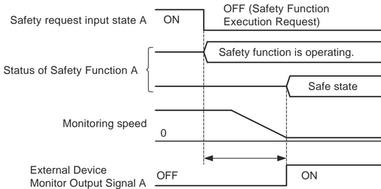
**Fig. 162: Operation Timing When Pc01.0 = 1 (Output Condition = Safe State)**
