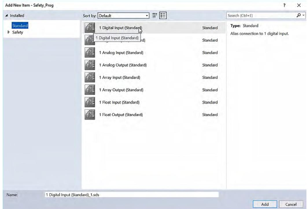
Fig. 126: TwinCAT 3 - Add Digital Input as Alias Device in TwinSafeGroup1
