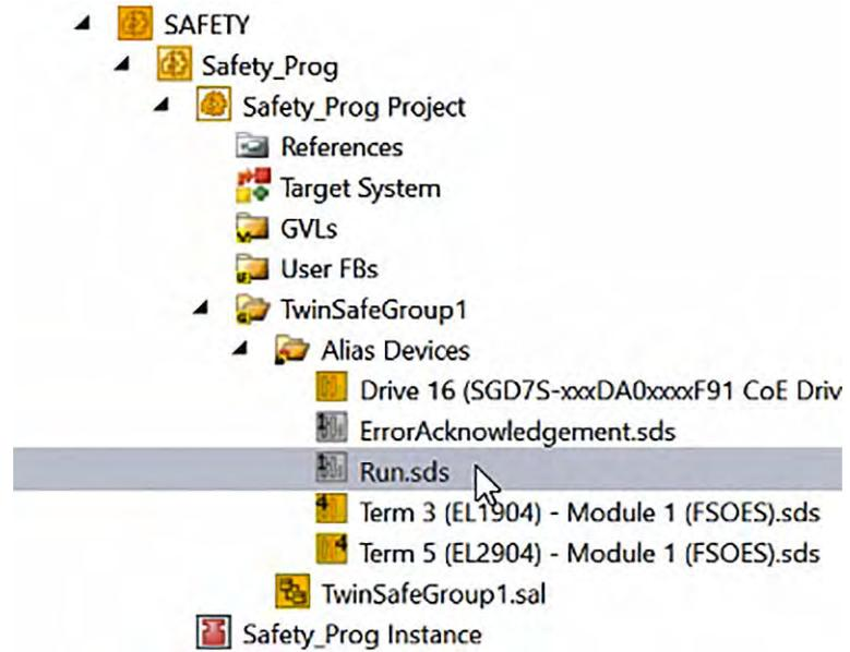
Fig. 104: TwinCAT 3 - Run Alias Device in Solution Explorer
