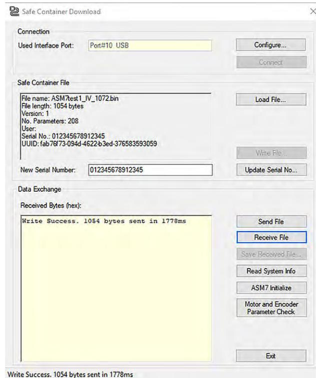
Fig. 4: Safe Container File Sending Completed
