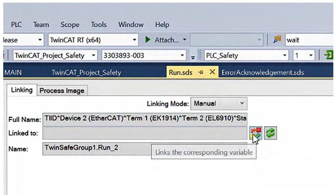
Fig. 105: TwinCAT 3 - Run - Link Button
