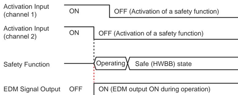
Fig. 165: EDM output behaviour of SGD7S-OSB01A
