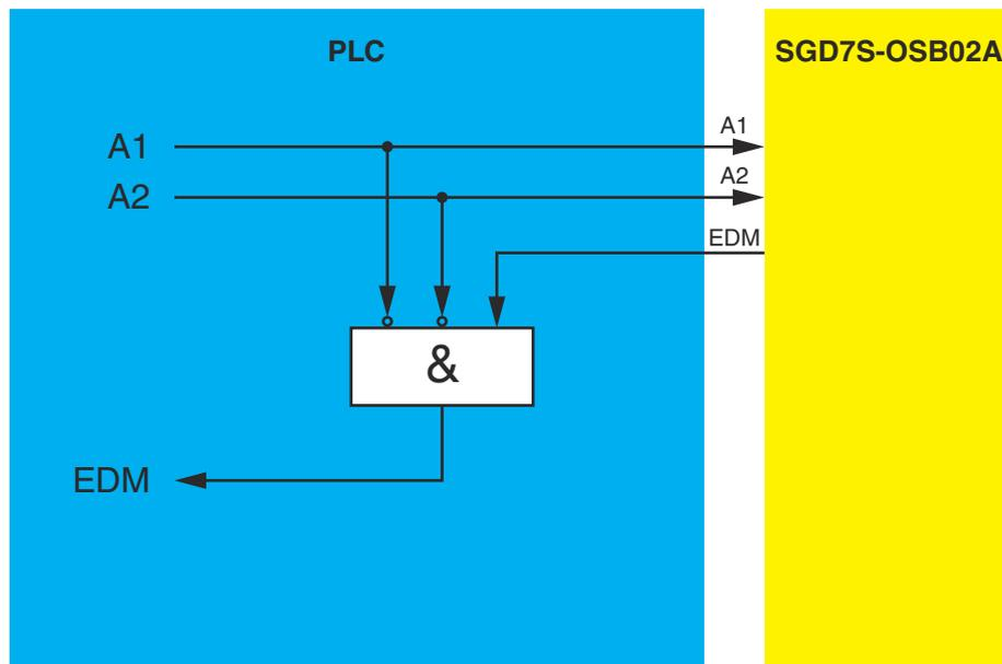
Fig. 166: Change behaviour of SGD7S-OSB01A/OSB02A to SGD7S-OSA01A
