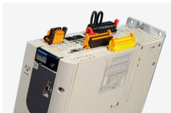
Sigma-7 safety cards integrate seamlessly into the Servopack. Therefore, both safe and non-safe axes have the same dimensions resulting in easier planning and maximum flexibility.
