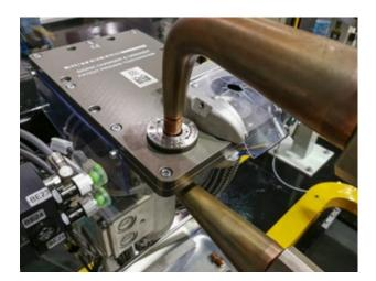
The automatic Tip Dresser and Tip Changer, is used in case of a fully automated workstation, where the electrode dressing and electrode change is performed automatically. The electrodes are placed in a magazine next to the dressing unit and the electrodes on the gun are replaced by an automatic extraction and replacement system.
