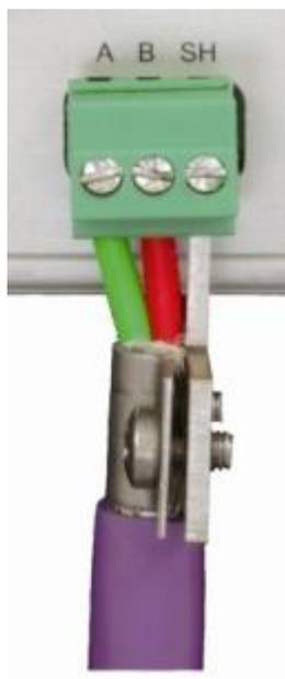
It is recommended to use the supplied ground clip to attach the cable shield to the screw connector, for easier shield connection and better strain relief.
