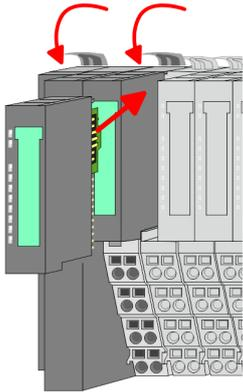
9. Plug again the electronic module, which you have removed before.
