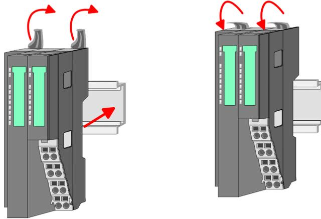
2. Turn the locking lever upwards, place the bus coupler at the mounting rail and turn the lever downward.
