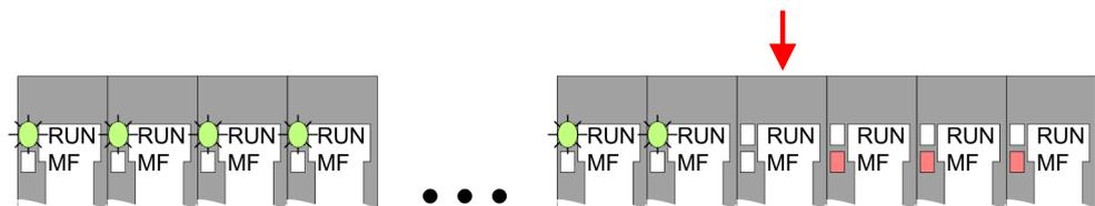
**Behaviour:** After PowerON all of the RUN LEDs up to the defective module are flashing. With all following modules the MF LED is on and the RUN LED is off.
