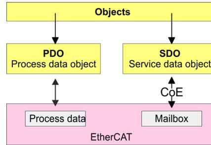
**PDO** PDO means **P**rocess **D**ata **O**bject. Process data may be transferred during run-time by means of PDOs. Here the Inputs respectively outputs are directly addressed within the frame. More concerning the process data transfer during run-time may be found in the manual of your EtherCAT master.
