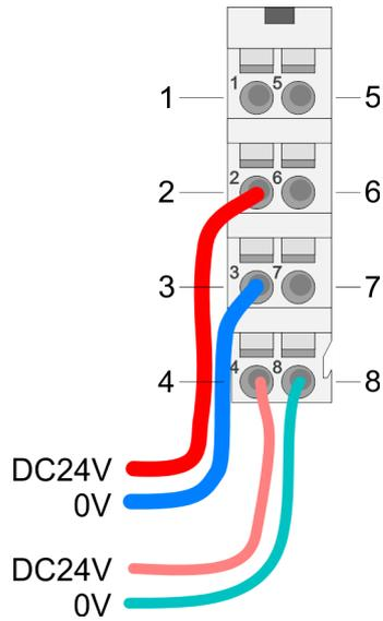
For wires with a core cross-section of 0.08mm<sup>2</sup> up to 1.5mm<sup>2</sup>.
