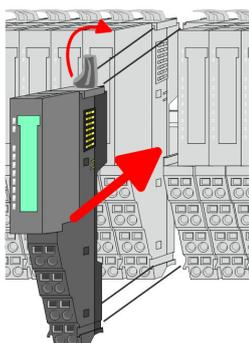
7. To mount the module put it to the gap between the both modules and push it, guided by the stripes at both sides, to the mounting rail.
