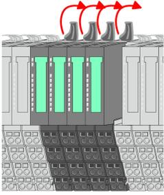
**4.** Turn all the locking lever of the module group to be exchanged upwards.
