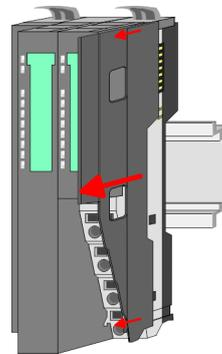
1. Before mounting the periphery modules you have to remove the bus cover at the right side of the bus coupler by pulling it forward. Keep the cover for later mounting.
