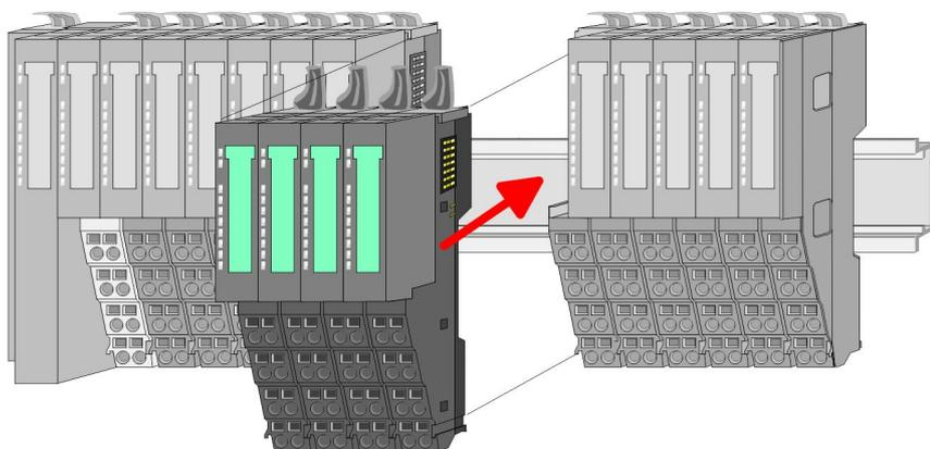
5. ▶ For mounting turn all the locking lever of the module group to be mounted upwards.
