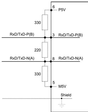
**i** The PROFIBUS line is to be terminated with its ripple resistor. Please consider to terminate the last participants on the bus at both ends by activating the terminating resistor.
