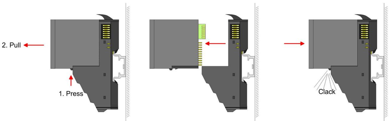
1. ➔ For the exchange of an electronic module, the electronic module may be pulled forward after pressing the unlocking lever at the lower side of the module.
