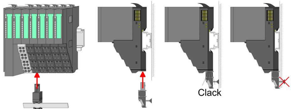
➔ The shield bus carrier (available as accessory) serves to carry the shield bus to connect cable shields. The shield bus carrier is mounted underneath the terminal of the terminal module. With a flat mounting rail for adaption to a flat mounting rail you may remove the spacer of the shield bus carrier.
