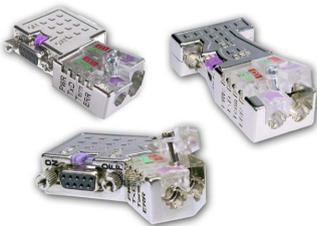
In PROFIBUS all participants are wired parallel. For that purpose, the bus cable must be feed-through. Via the order number 972-0DP10 you may order the bus connector "EasyConn". This is a bus connector with switchable terminating resistor and integrated bus diagnostic.
