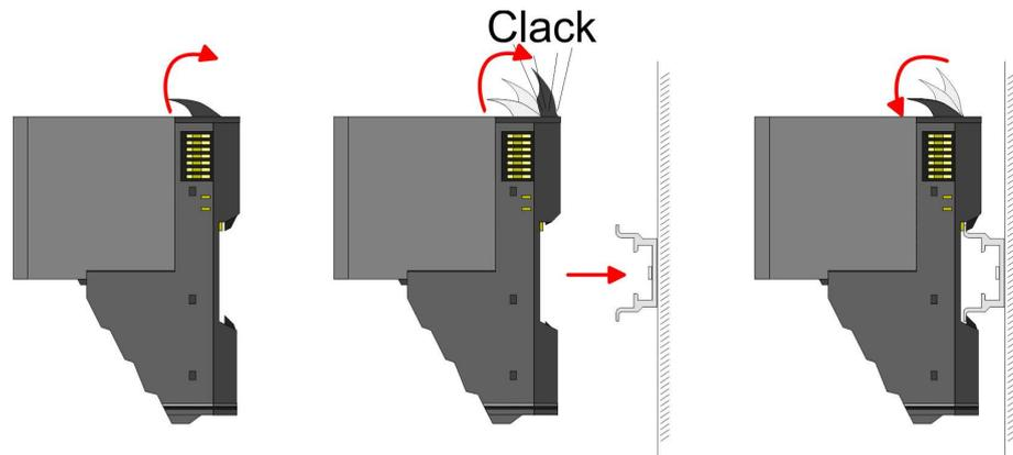
For the exchange of a electronic module, the electronic module may be pulled forward after pressing the unlocking lever at the lower side of the module. For installation plug the electronic module guided by the strips at the lower side until this engages audible to the terminal module.
