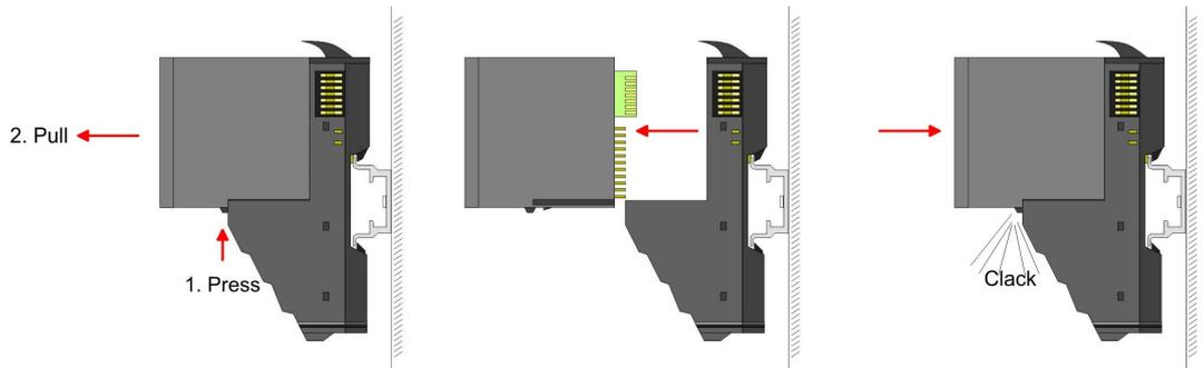
2. ➤ For the exchange of a electronic module, the electronic module may be pulled forward after pressing the unlocking lever at the lower side of the module.
