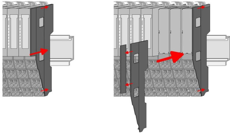
3. After mounting the whole system, to protect the backplane bus connectors at the last module you have to mount the bus cover, now. If the last module is a clamp module, for adaptation the upper part of the bus cover is to be removed.
