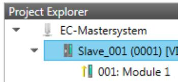
In a *Hot Connect group* several slave stations can be located, which must only optional be available at the EtherCAT bus. So you have the possibility to take or add pre-configured sections from the traffic before starting the system or during the operation. This can be done by disconnecting/connecting the communication path or enabling/disabling the participant.
