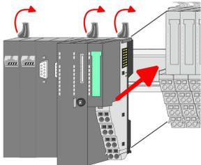
7. ➤ To mount the CPU put it to the left periphery module and push it, guided by the stripes, to the mounting rail.
