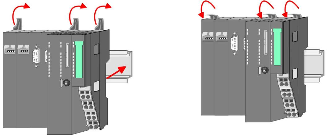
2. Turn the locking lever upwards, place the CPU at the mounting rail and turn the lever downward.
