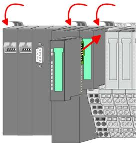
9. ➤ Plug again the electronic module, which you have removed before. For installation plug the electronic module guided by the strips at the lower side until this engages to the terminal module.
