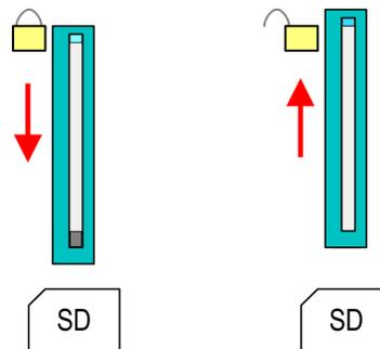
To remove, slide the sliding mechanism up again and push the storage media against the spring pressure until it is unlocked with a click.
