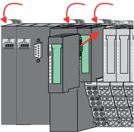
**9.** Plug again the electronic module, which you have removed before. For installation plug the electronic module guided by the strips at the lower side until this engages to the terminal module.
