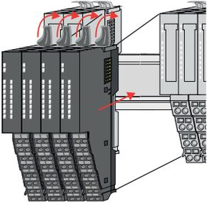
6. ➤ To mount the module group put it to the gap between the both modules and push it, guided by the stripes at both sides, to the mounting rail.
