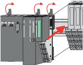
**7.** To mount the CPU put it to the left periphery module and push it, guided by the stripes, to the mounting rail.
