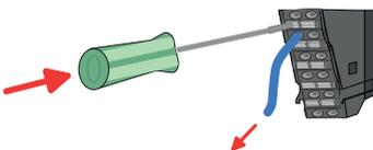
The wire is to be removed by means of a screwdriver with 2.5mm blade width.
