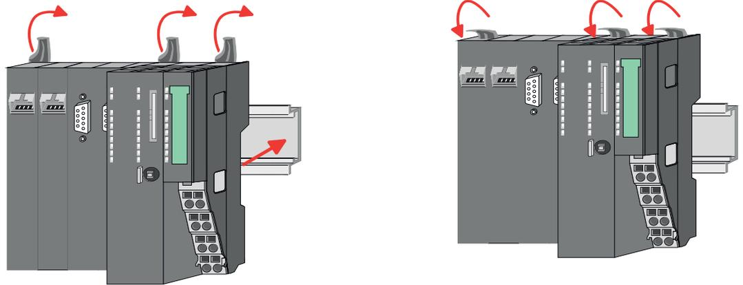
2. Turn the locking lever upwards, place the CPU at the mounting rail and turn the lever downward.
