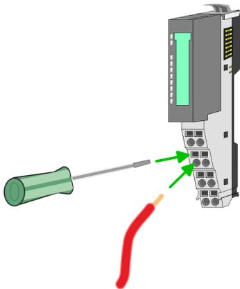
1. Insert a suited screwdriver at an angle into the square opening as shown. Press and hold the screwdriver in the opposite direction to open the contact spring.
