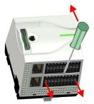
**8.** Remove the connectors, which are not necessary at the CPU.
