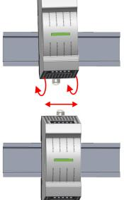
**4.** Move the power supply on the profile rail at its position.
