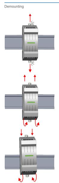
1. Use a screwdriver to pull the locking levers of the power supply outwards until these engage audible.
