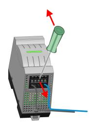
By means of a screwdriver there is the possibility to remove the connectors e.g. for module exchange with a fix wiring. For this each connector has indentations for unlocking at the top. Unlocking takes place by the following proceeding:
