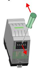
1. Remove the connectors, which are not necessary at the power supply.
