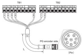
Figure 9 Wiring PG Encoder Cable
