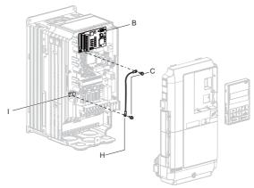
Figure 5 Connect the Ground Wire
