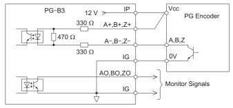
Figure 15 Open-Collector Outputs for the Interface Circuit
