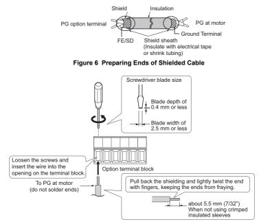
Figure 7 Preparing and Connecting Cable Wiring
