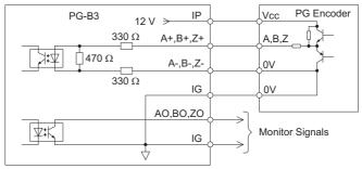
Figure 14 Complementary Outputs for the Interface Circuit
