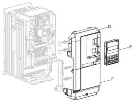
Figure 11 Replace the Front Covers and Digital Operator
